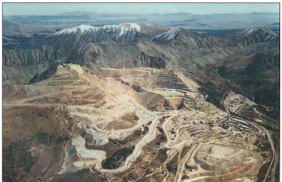
Figure 13.14 Climax molybdenum mine near Leadville, Colorado. At an altitude of approximately 11,000 feet, the mine was first developed as an underground mine around World War I, when molybdenum became recognized as a useful alloy to harden steel, and for a time accounted for a majority of global production of this mineral. Open-pit operations began in the early 1970s.
