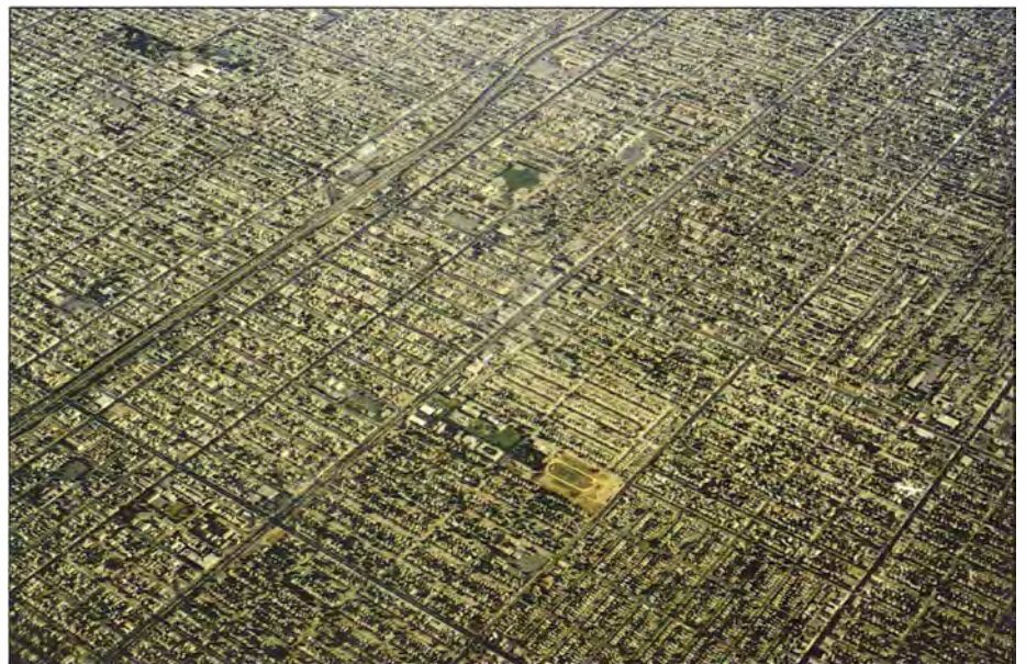
Figure 14.1 Rectilinear residential tracts in southwest Los Angeles, reflecting a sense of order, rationality, and expedience, recall the repetitive gridiron plans of new towns in the 19th century. Here, even the modern freeway, Interstate 110, south of its intersection with Florence Avenue (at left margin), cuts southward through the area in alignment with the grid.
