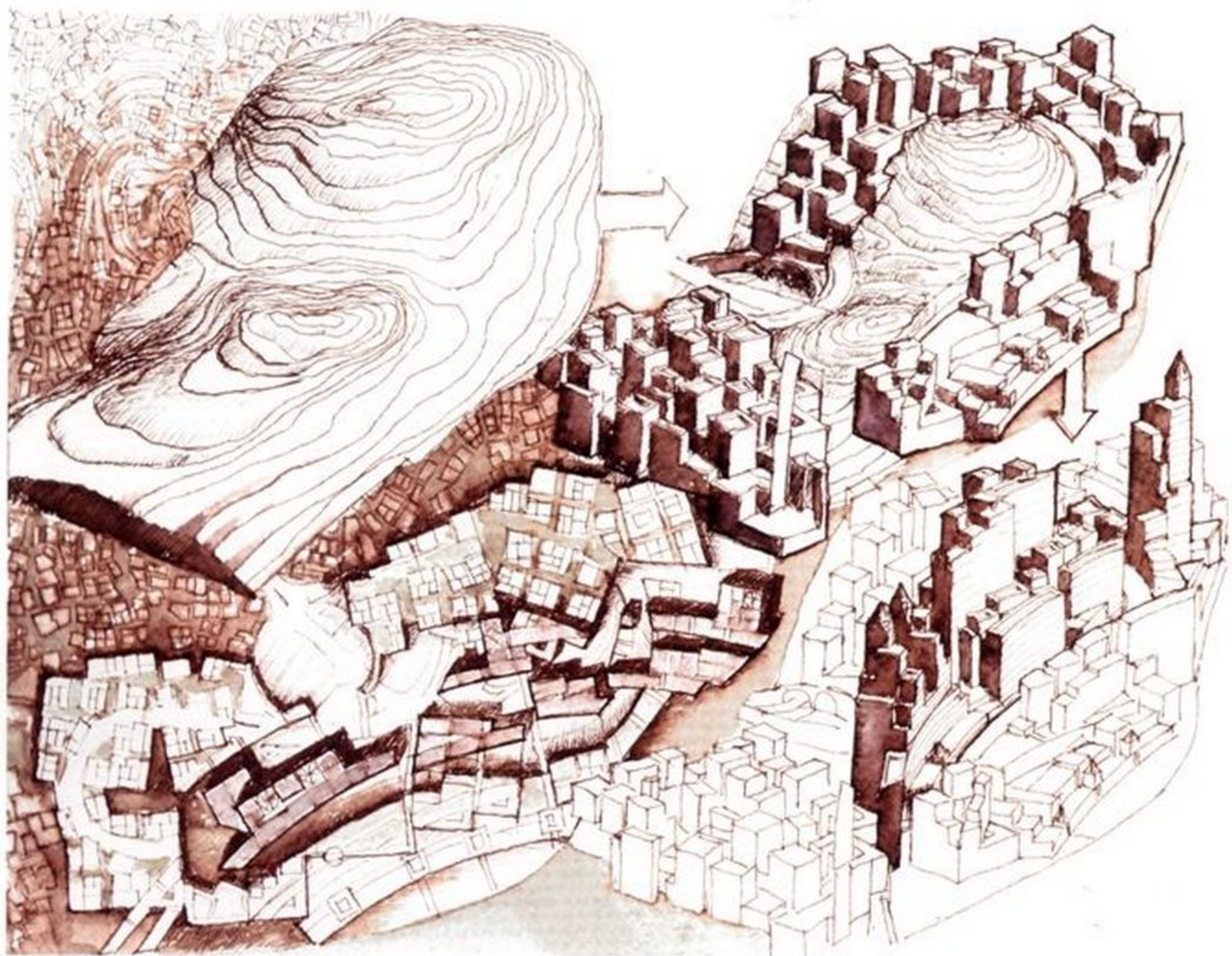
Jabal Omar housing development, Makkah. An axonometric drawing showing how the slopes were used to best advantage to ensure views towards the Haram al-Sharif and the Ka'bah. Rasem Badran identified the social diversity of the overall structure. Shown on the left is the living cluster.
