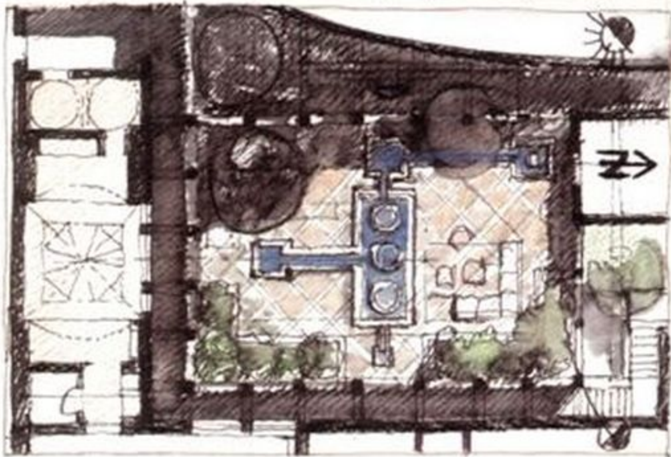
Above and right Al-Talhouni residence, Amman, Jordan. The orientation of each courtyard must be carefully adjusted to permit maximum airflow, with sectional proportions adjusted accordingly. The carved water fountains (right), designed by Rasem Badran's late father, Jamei Badran, serve an environmental purpose as well, cooling the air.
