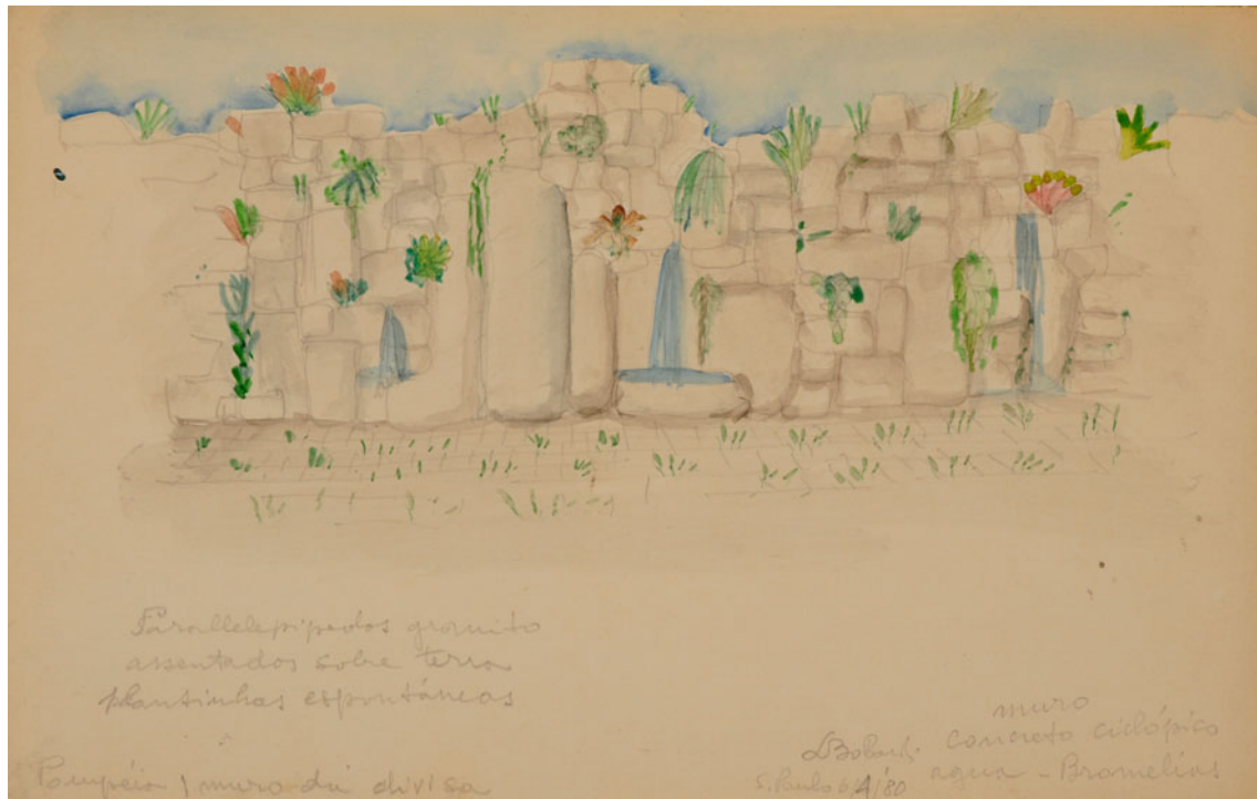
Fig. 3.2 Lina Bo Bardi's elevation of a broken wall recomposed into a new wall made up of "architectural spoils" merged with plants, for the SESC Pompeia factory in São Paulo, 1977 (Instituto Lina Bo e PM Bardi)
