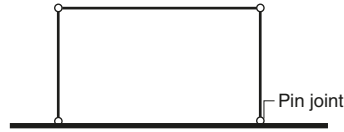
Structural model (stability provided by structure elsewhere in plan)
