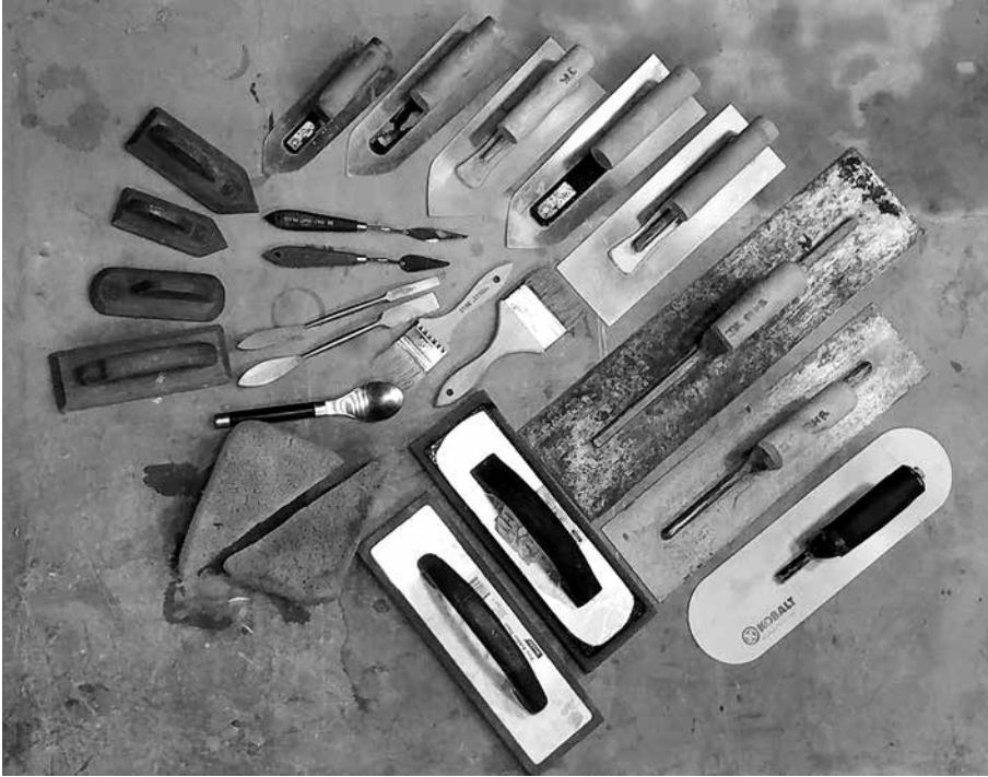
6-26. A variety of floats, trowels, and tools for finishing plaster.
