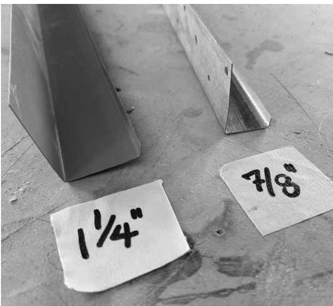
6-13. Casing bead profiles.
