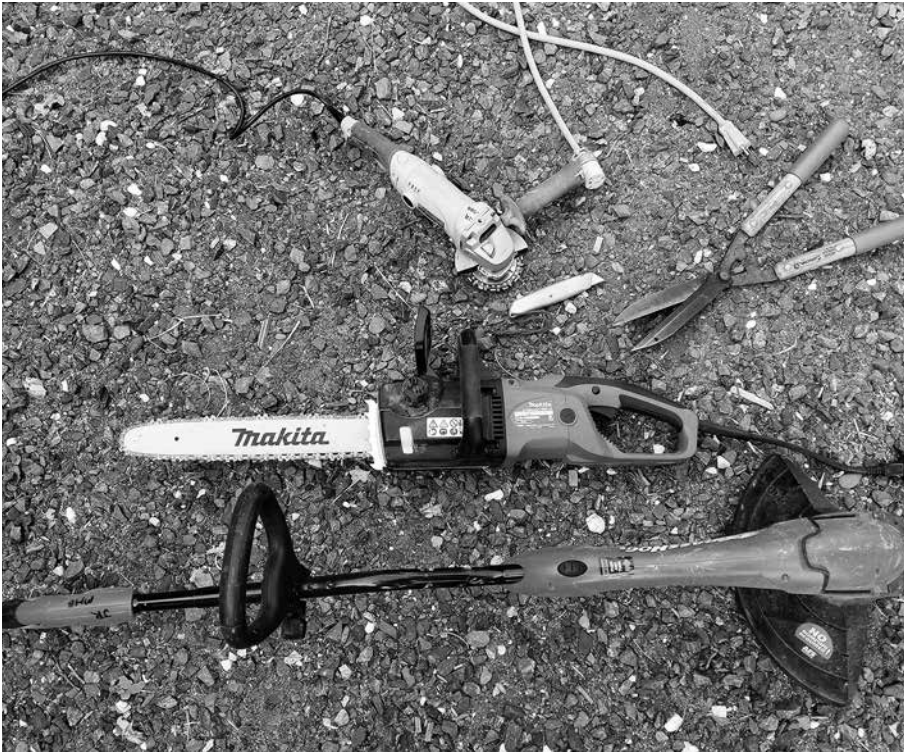
5-20. Tools for trimming bale walls.
