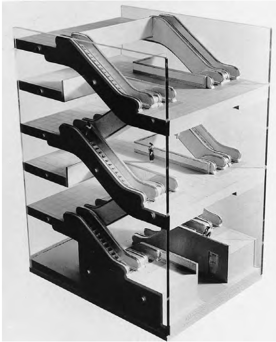
Figure 11.3a Escalator design: Concept model for Harrods' escalators, late 1930s (courtesy of Mr M. Al Fayed, Chairman of Harrods Ltd)
