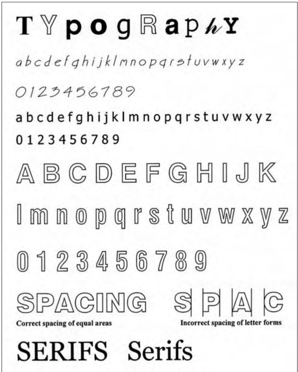
FIGURE 4.4 Examples of various typefaces in current use.
