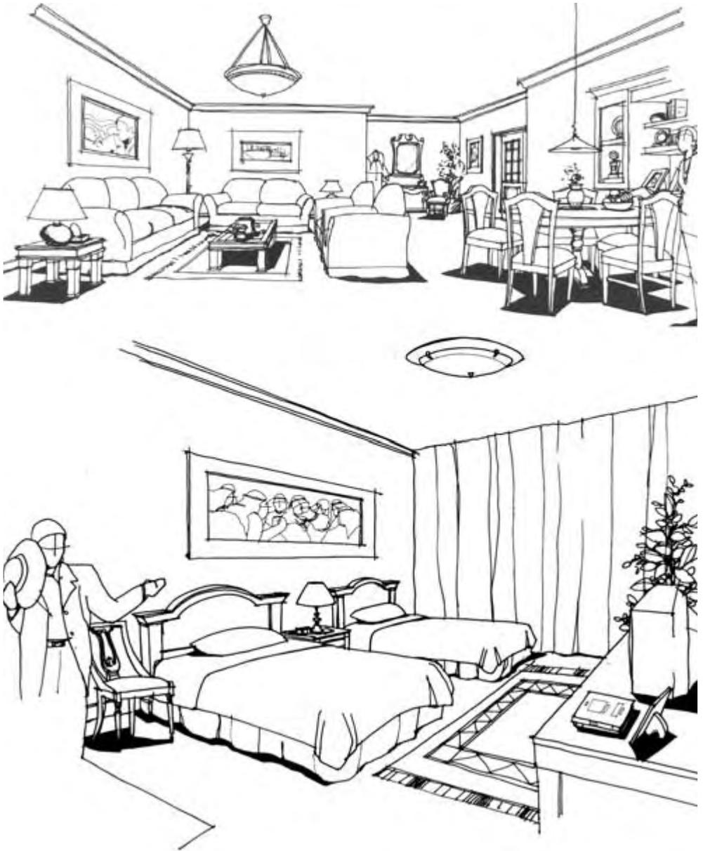
**FIGURES 4.19** Two examples of one-point perspective. (Drawings by Ibtisam Sharbaji, Kubba Design)
