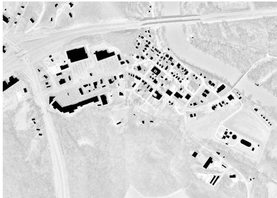
Figure 7-4 Figure-ground diagram showing building “footprints” superimposed on a vertical aerial photograph. This mapping technique facilitates a visual assessment of urban “texture” – an important contextual attribute. Source: The HOK Planning Group.
