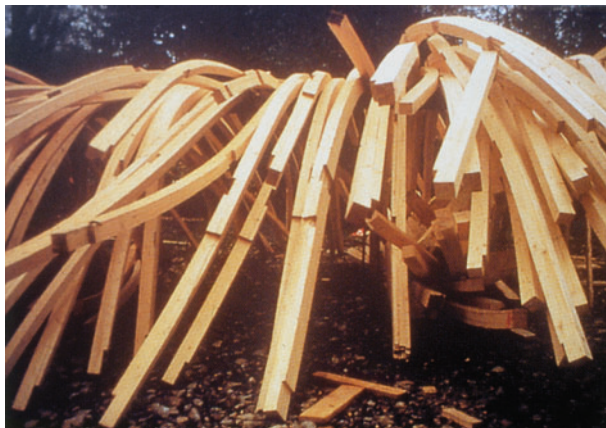
Figure 12.8 Prefabricated, strongly doubly curved glulam beams ready for transport to site
