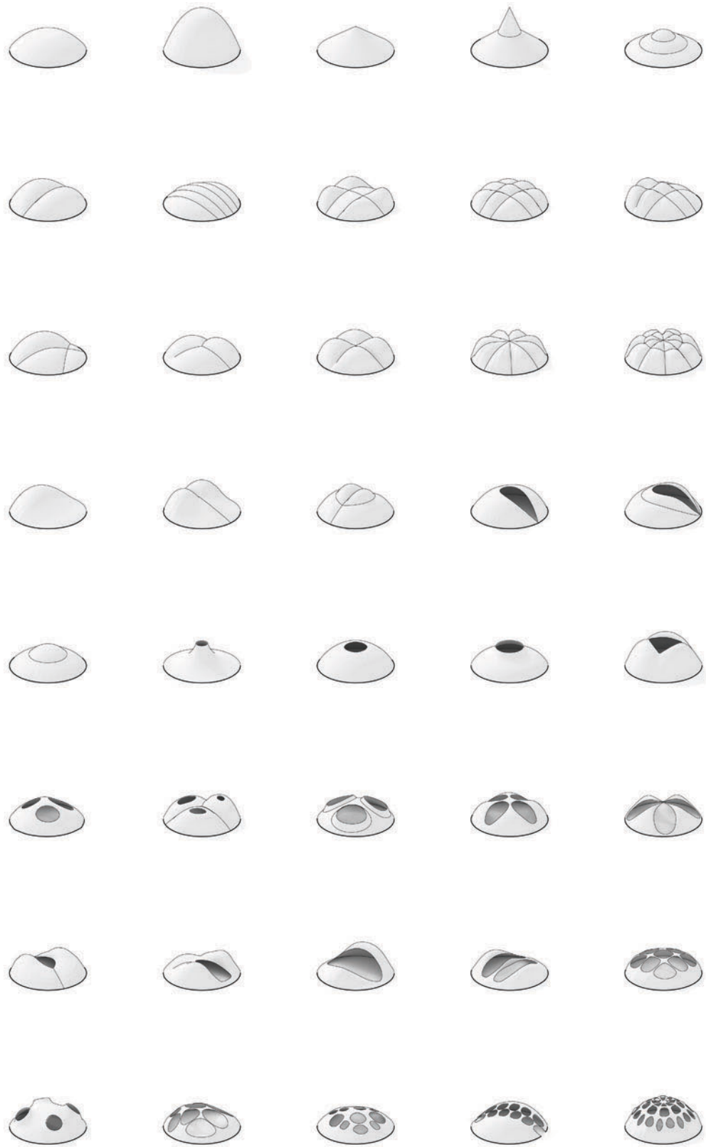
Figure 1.5 Compression-only shell geometries supported on a circular plan found using thrust network analysis
