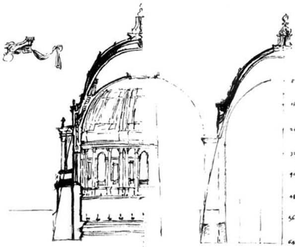
Figure 4.2 St Paul's Cathedral, London. Sketch of Hooke's catenary superimposed on a proposed section of the dome
