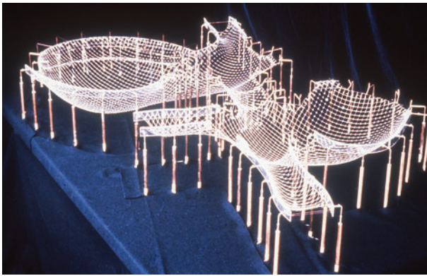
Figure 4.14 The finished hanging-chain model of the Multihalle surveyed using photogrammetry to determine its precise geometry
