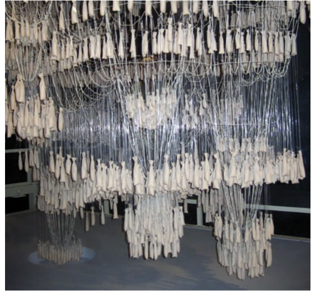
Figure 4.6 Reproduction of Gaudí's hanging model for the crypt of Colònia Güell, Barcelona
