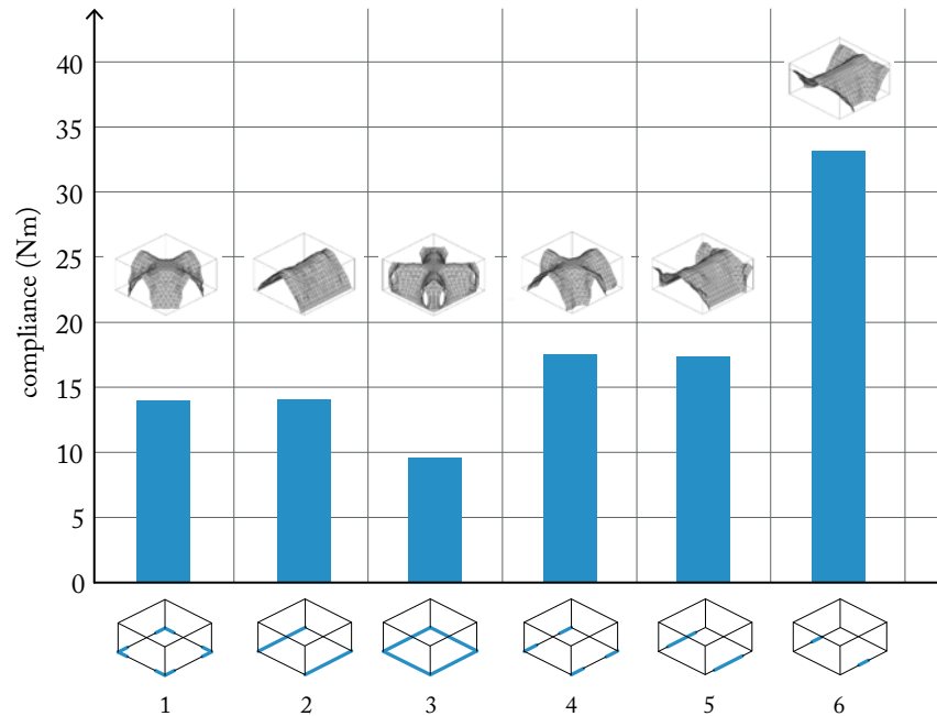
Figure 17.11 Diagrams illustrating the cuboidal design space and structural systems of models 1–6: bold lines indicate the supports of the structure
