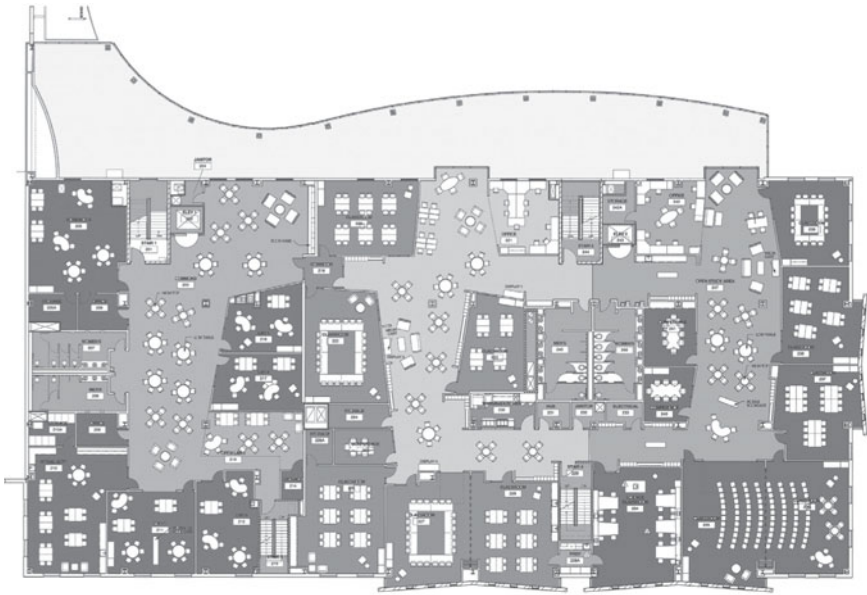
Figure 8. Cristo Rey High School, Minneapolis, MN. Second floor plan illustrating the translation of the Learning Suite pattern with three small learning communities each containing learning studios and suites surrounding collaborative breakout areas (courtesy of Fielding Nair International, LLC).
