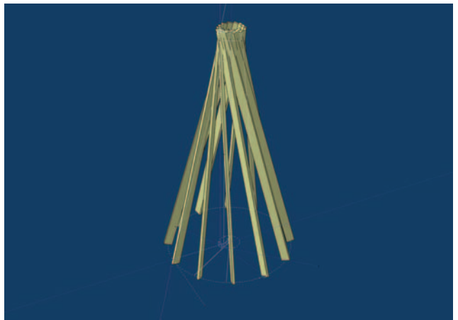
▲ 4.13 Steep RF with 12 beams. (Drawing: Chris Dunn.)
