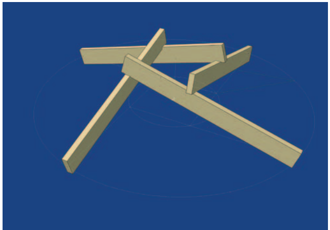
▲ 4.5 RF with four beams and small inner radius. (Drawing: Chris Dunn.)
