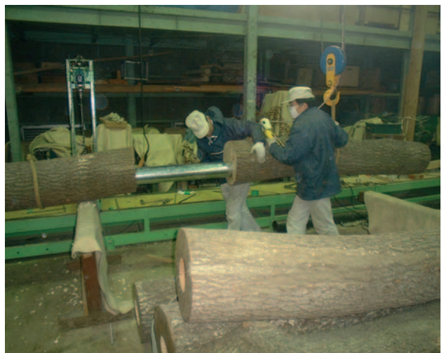
▲ 7.4 Steel core reinforcement. (Photo: Kazuhiro Ishii.)
