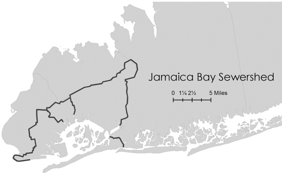
Figure 4-3. The sewersheds of Jamaica Bay. This map shows the areas that drain to the four wastewater treatment plants managed by the City of New York, which mainly, but not entirely, follow the topographic watersheds. Two other plants treat sewage from Nassau County (not shown). Courtesy of Joy Cytryn of Hunter College, City University of New York.
