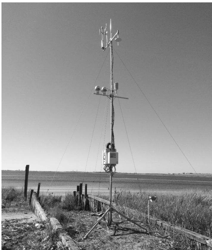
Figure 7-5. A meteorological mast deployed on the north side of Black Bank near the National Park Service visitor contact station at the Jamaica Bay Wildlife Refuge. Representative measurements are shown in figure 7-6. Courtesy of Christopher J. Zappa of Lamont-Doherty Earth Observatory, Columbia University.
