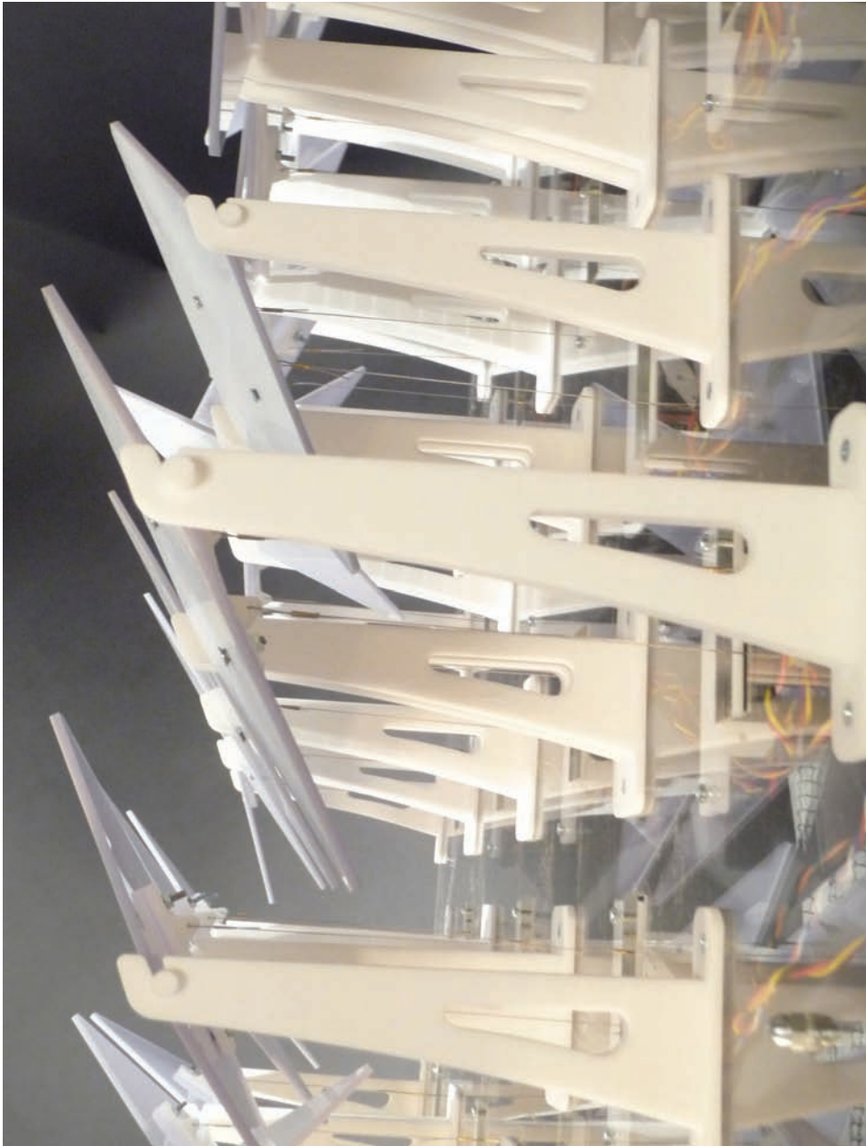
Adaptive Fa[CA]de was presented at Digital Hinterlands, an exhibition at Arup Phase 2 Gallery in London as part of Design Week in 2009. The kinetic prototype consisted of a grid of twenty-five individually controlled panels. A side view of the prototype shows the 3D-printed components that hold the panels, allowing them to tilt along their x-axis. (Courtesy Marilena Skavara)
