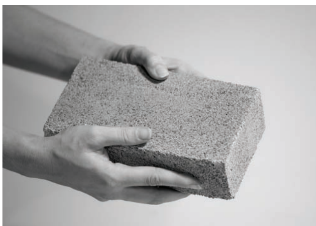
Image of a full scale Biomanufactured Brick. (Courtesy Ginger Krieg Dosier)
