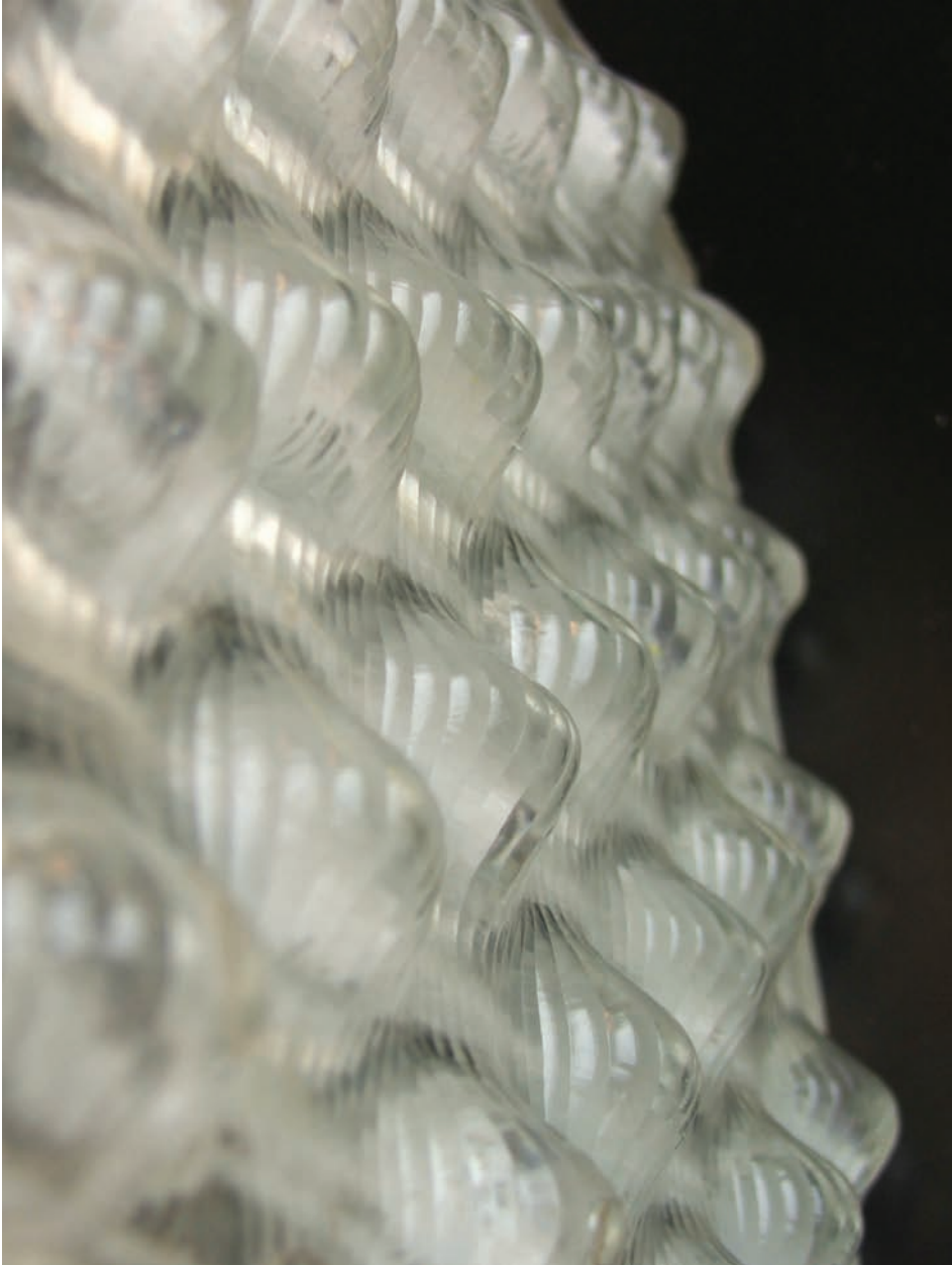
Latent Shift is part of ongoing research on the use of phase change material in architectural application. Prototypes developed include continuous core panels that isolate the PCM from its polyester substrate, allowing the material to visually exhibit shifting and variable properties in response to temperature changes. (Courtesy Rashida Ng and Sneha Patel)
