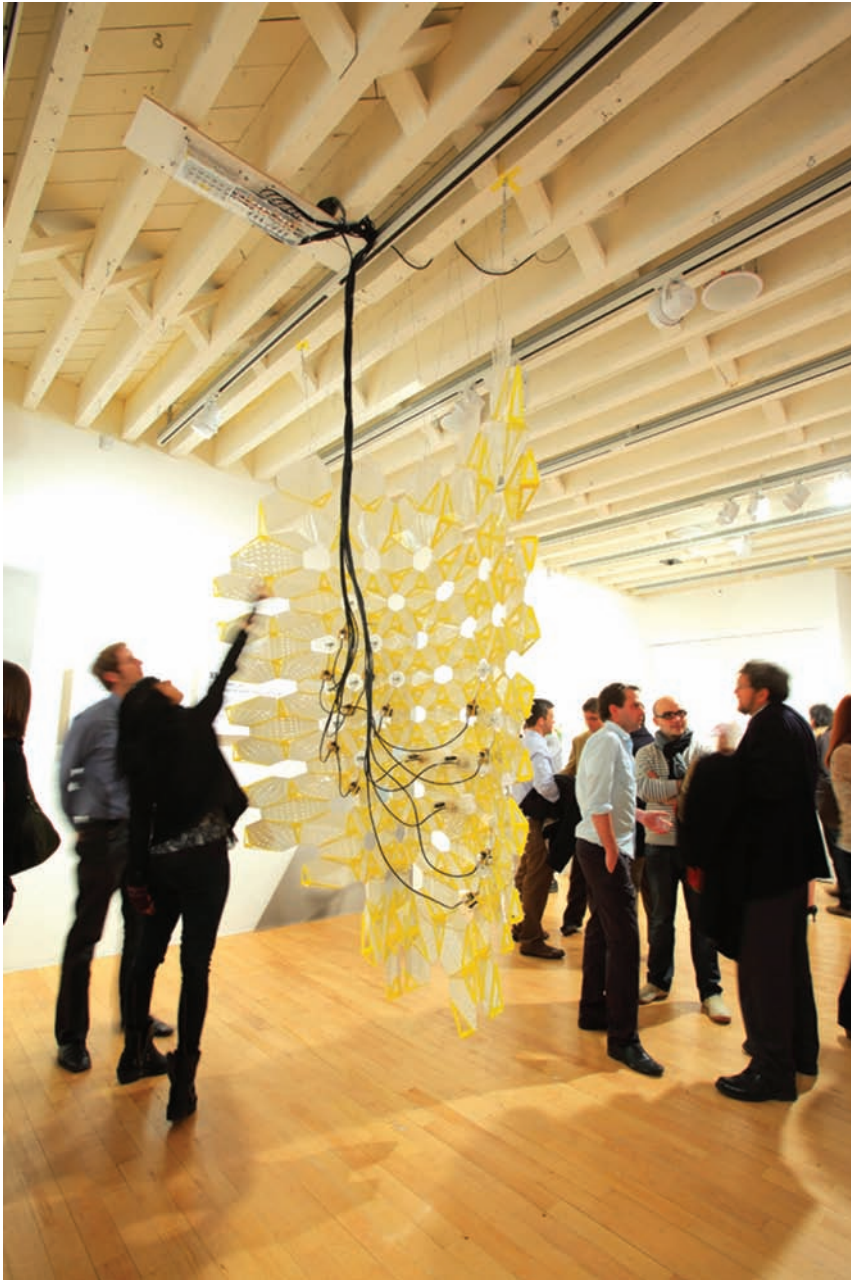
Xeromax Envelope is a quarter-scale experiment for a responsive building envelope calibrated and tuned to its environment. Part robotic structure, part experimental interface, and part microclimatic machine, it registers energy cycles and interactions over time while harvesting solar energy and protecting the building from the local climate. (Courtesy Future Cities Lab)
