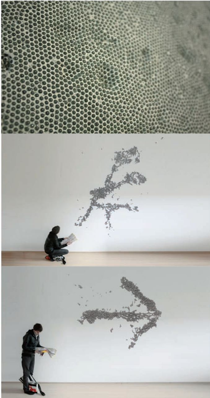
BlingCrete. Close-up view of mockup (glass and concrete) in random pattern, green matrix (Photo: Boris Trenkel); Magnetic Positioning of Concrete [computer simulation]. (Courtesy Klussman, H., Klooster, T., and Winkler, C.)
