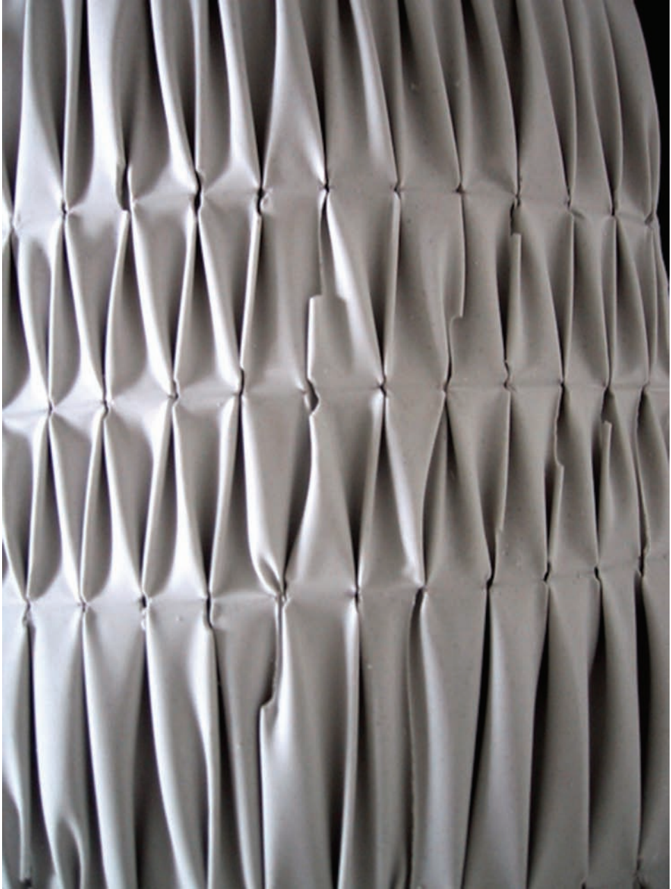
Plaster cast detail, Smocking v3; Smocking explores the potential of a pleating technique on a fabric formed concrete surface, a manifestation of an equilibrium reached between the surface tension and omni-directional hydrostatic pressure. (Courtesy Kentaro Tsubaki)
