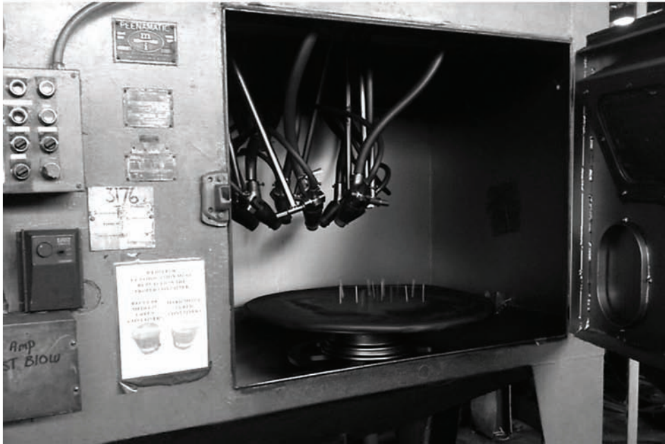
Designed Disorder includes ongoing research into CNC shot peen forming. This fabrication process offers the unique opportunity to privilege imperfection or variation when paired with high precision. Images illustrate Peening Jig Prototypes and Numerically Controlled Peening Tools. (Courtesy Phillip Anzalone, Brigette Borders, and Kerri Henderson)
