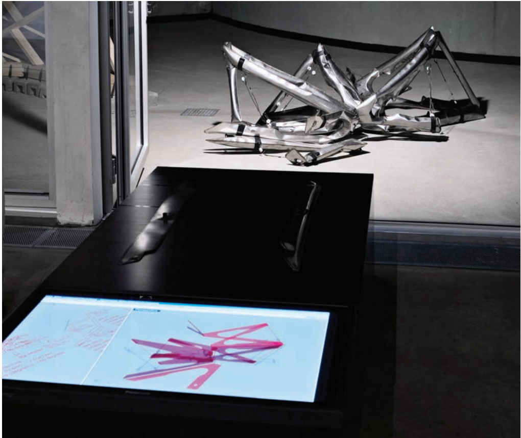
The digital model co-exists with the material artifact continually being re-informed from the material as it is selectively inflated. The digital model therefore reflects and uses the as-existing condition from which to determine further design moves rather than relying upon an idealized condition. (Courtesy CITA)
