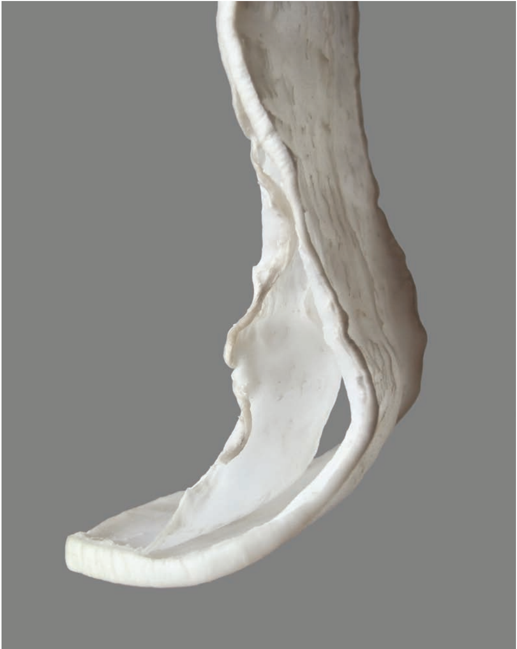
This work is part of ongoing PhD research conducted at the Tokyo University of the Art in the development of architectural forms based on nanotechnology and 3D textiles. Experiments in nano-textiles include studies of moisture content (20 percent shown) and corresponding geometric configurations. (Courtesy Klaudia Biala)
