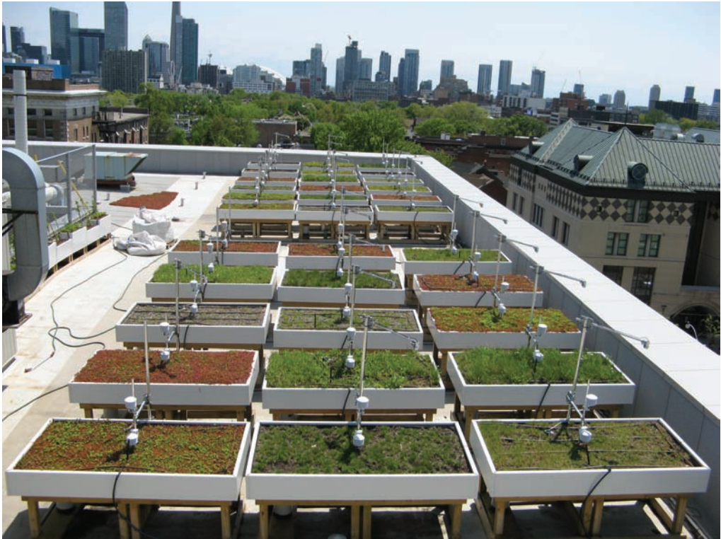
GRITLab In-situ View of green roof instrumentation at the John H. Daniels Faculty of Architecture, Landscape and Design—University of Toronto. (Courtesy Liat Margolis)
