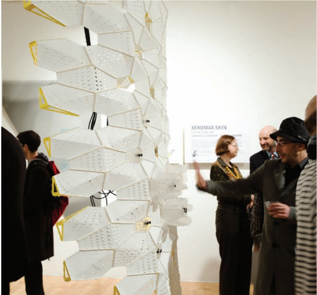
Xeromax Envelope is proposed as a second skin for an existing building and becomes a register of present and forecasted conditions. The model weaves ultra-thin custom actuators, arrays of light, and proximity sensors through the extent of the surface which transforms as it registers the changing conditions around it. (Courtesy Future Cities Lab)
