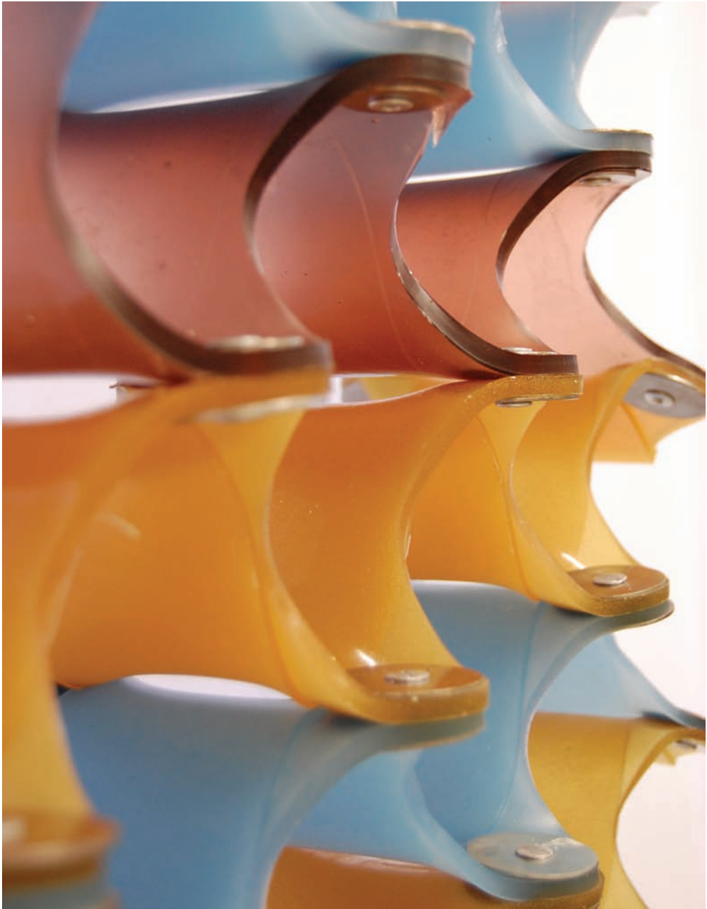
Gravity Screens (2010) Full scale gravity screen with different Shore elastomers. (Courtesy Omar Khan)
