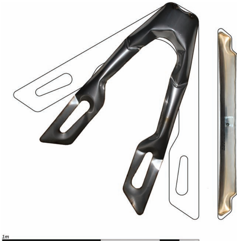
The material forming technique of free-form inflation contributes significantly to the component attributes, causing them to deviate with varying degrees from the initializing representations used to cut the profiles. (Courtesy CITA)
