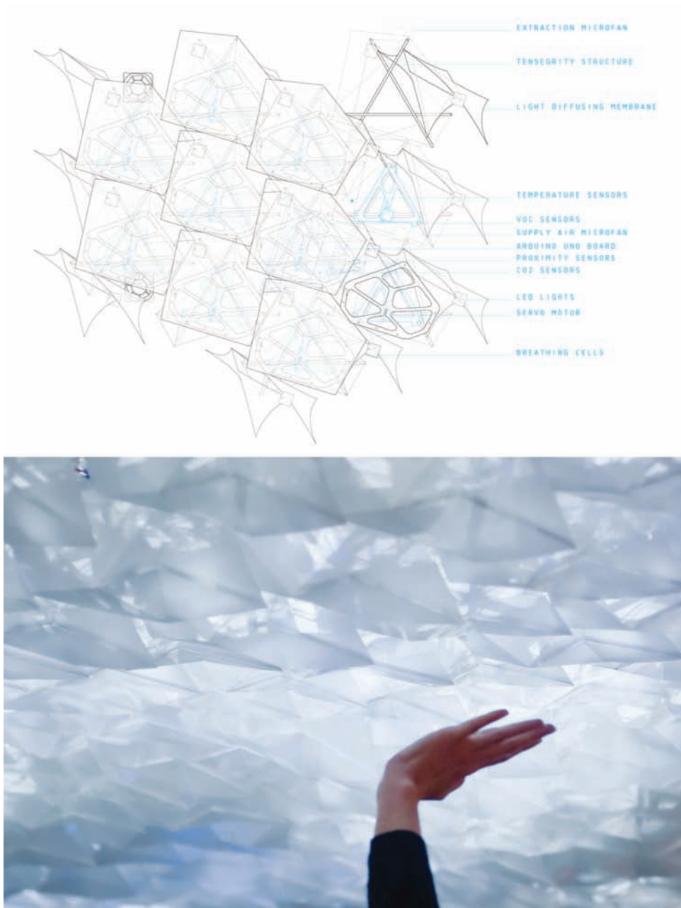
The Stratus Project is part of an ongoing body of research investigating the potential for kinetic, sensing and environment-responsive interior envelope systems. The top image is a plan of the Stratus component array and the bottom image presents The Stratus Project v1.0 prototype responding to occupant presence. (Courtesy RVTR)
