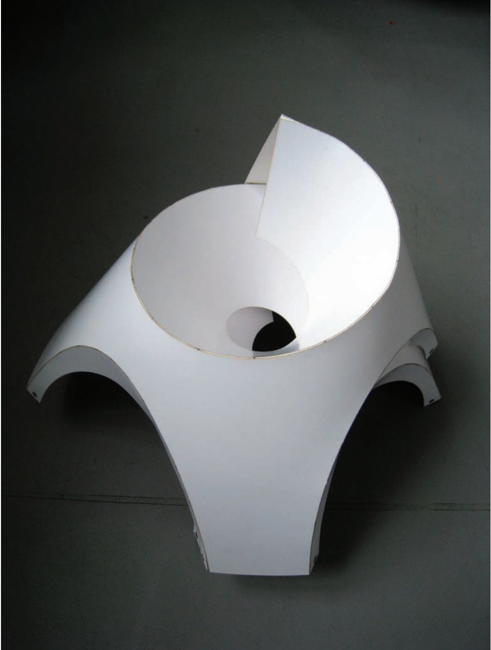
Physical prototype investigating a self-bracing creased developable surface. (Courtesy CITA)
