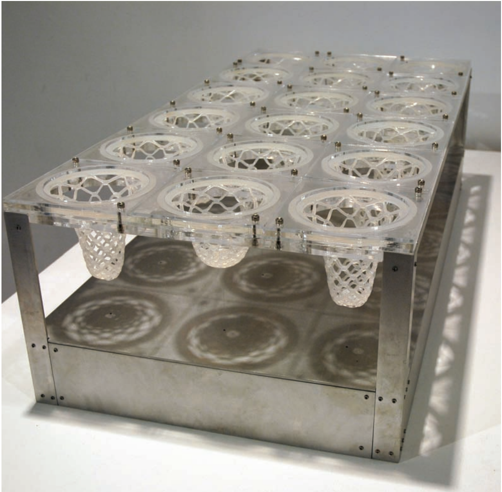
Columns Homeostat (2006) is a performative model to study the spatial performance of multiple columns. Different programs, like a cellular automata or prescribed choreography, can be run on the model. (Courtesy Omar Khan)
