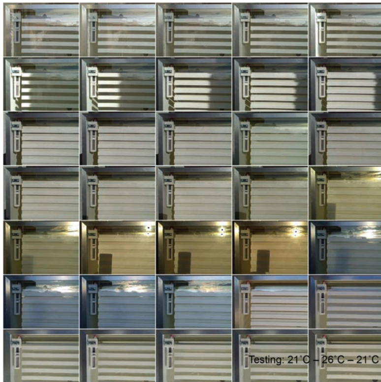
Testing of the SmartScreen III prototype over the course of a day, at temperatures ranging from 21 to 26 degrees Celsius. (Courtesy Decker Yeadon LLC)
