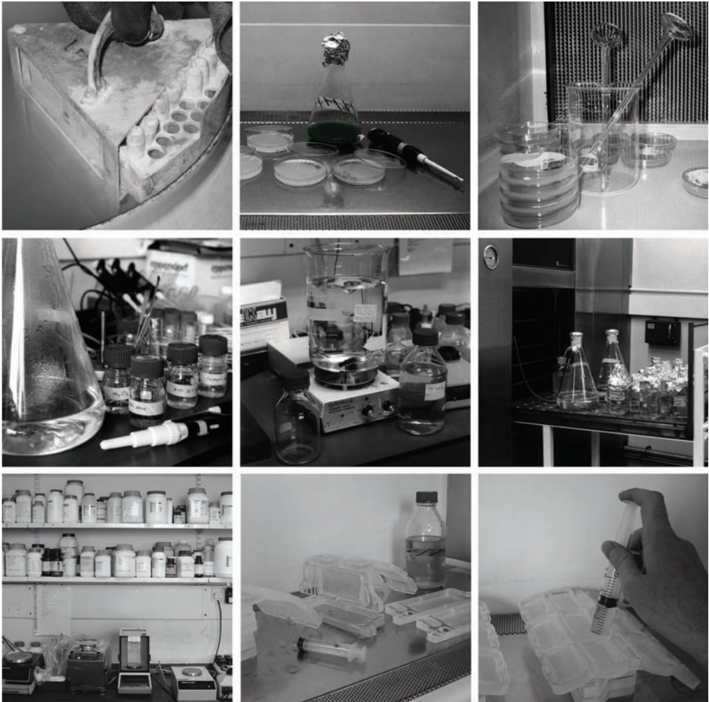
Process The preparation of Monitor Vessels and growth plates under sterile conditions at the UCL Department of Microbiology laboratory. The specific composition of the growth medium is tailored in order to target particular ambient microbial populations. (Courtesy Steve Pike)
