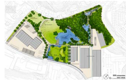
Behind the park design is an innovative and comprehensive water management concept. A rainwater canal is opened, the water returned to the surface, cleansed and released back into the Alna.
