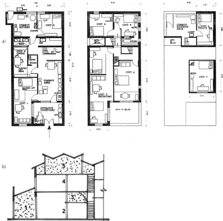
Figure 12. Densification in lilong housing. a) Floor plans after densification (source: D. Louise Morris, 1994). b) Front section after densification (source: sketch by the author).
