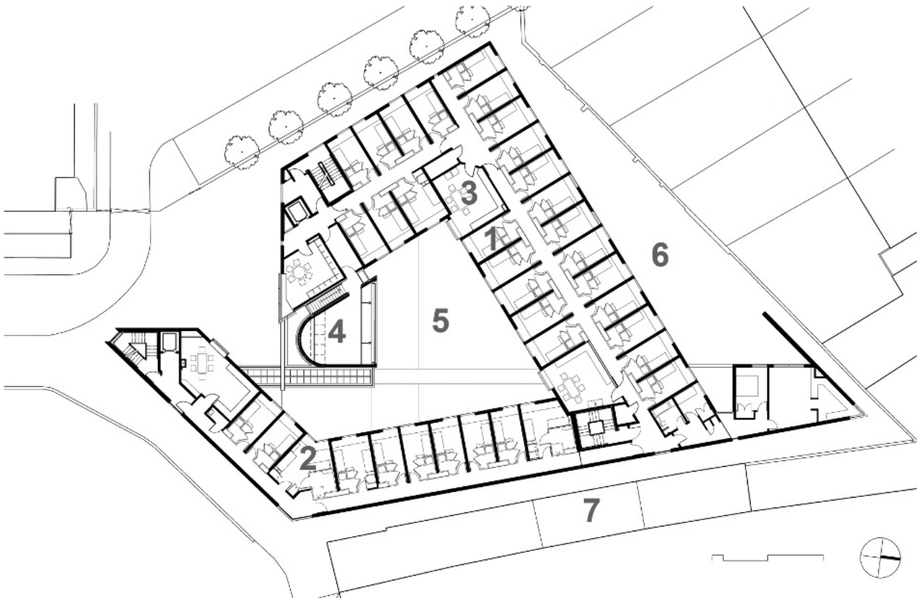
9.4 Generic type: student and key-worker housing with a corridor arrangement: Friendship House, London. Architects: MacCormac Jamieson Prichard. The corridor arrangement is wrapped around a courtyard to provide a focus for residents. 1, study bedroom; 2, study bedroom for disabled residents; 3, shared kitchen; 4, common room; 5, courtyard; 6, garden; 7, railway viaduct
