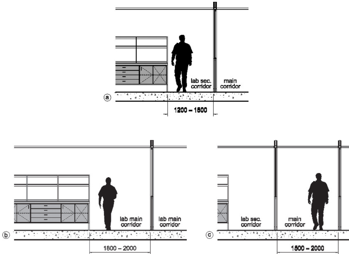
23.17 Aisle and corridor widths (a) at the ends of benches, additional means of circulation within the laboratory; (b) at the ends of corridors, single means of circulation within the laboratory; (c) general circulation
