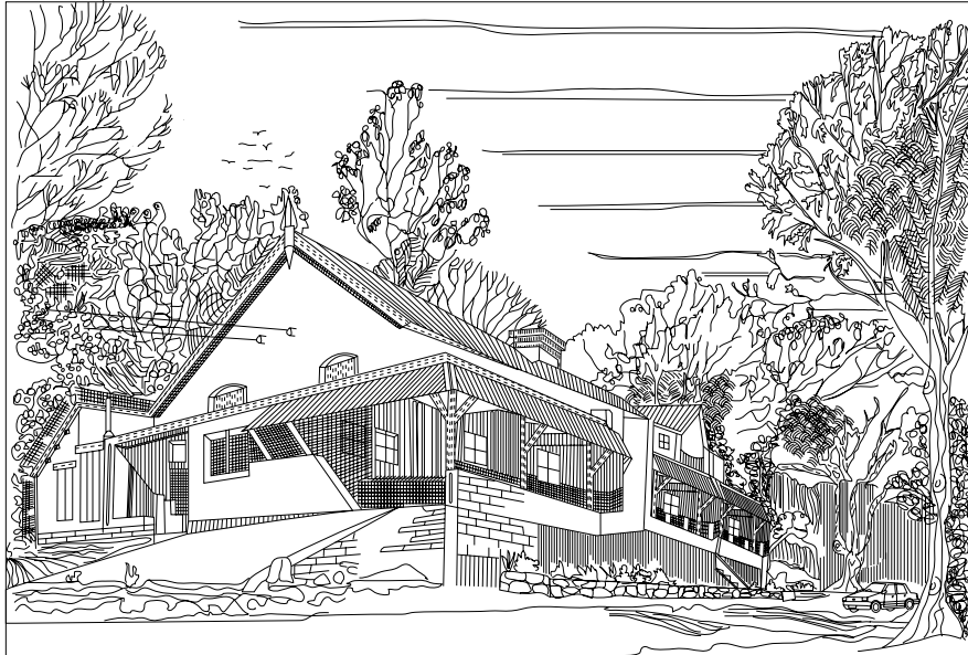
35.2 Colonial bungalow, Zomba, Malawi, with clerestory windows, high ceilings and deep shaded verandas, including one for the car. Drawing by the Rev'd D Brian Roy, RIBA
