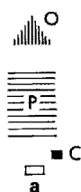
34.35 Bad organ arrangement. Key: o organ, c organ console, p people, ch choir, m minister, a altar
