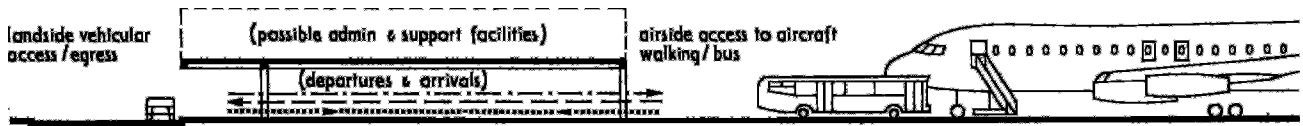
a Single-level terminal, generally applicable to small or domestic terminals Arrival and departure routes split horizontally as flow plan diagram 30.4
