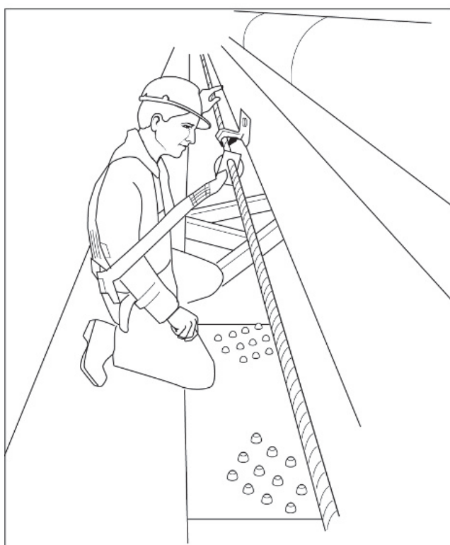
45.9 A continuous wire cable with harness-clip that rides through the anchor fixings (Latchways plc). a Fixing to a wall. b In use
