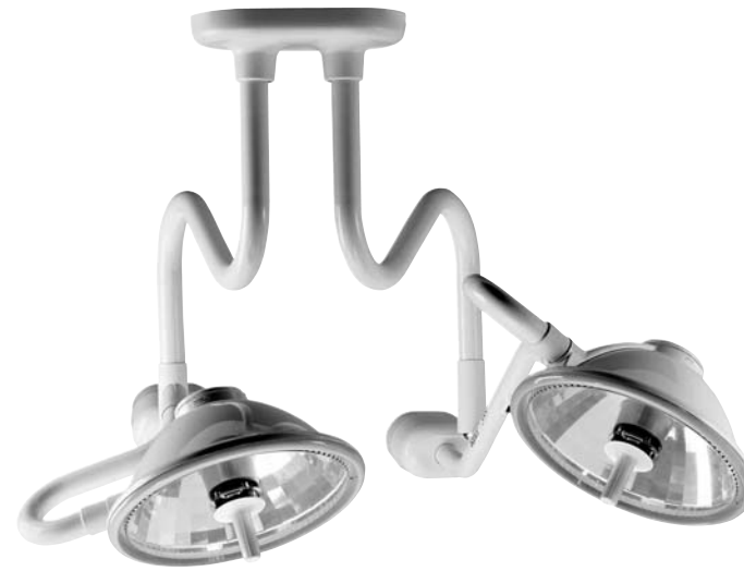
Figure 10-121. Dual halogen minor surgery light, Ritter® model 355; lamp has 4200K color temperature; provides 4000 fc at 36-inch focal length and 6200 fc at 24-inch focal length. (Photo courtesy: Midmark Corporation, Versailles, OH.)
