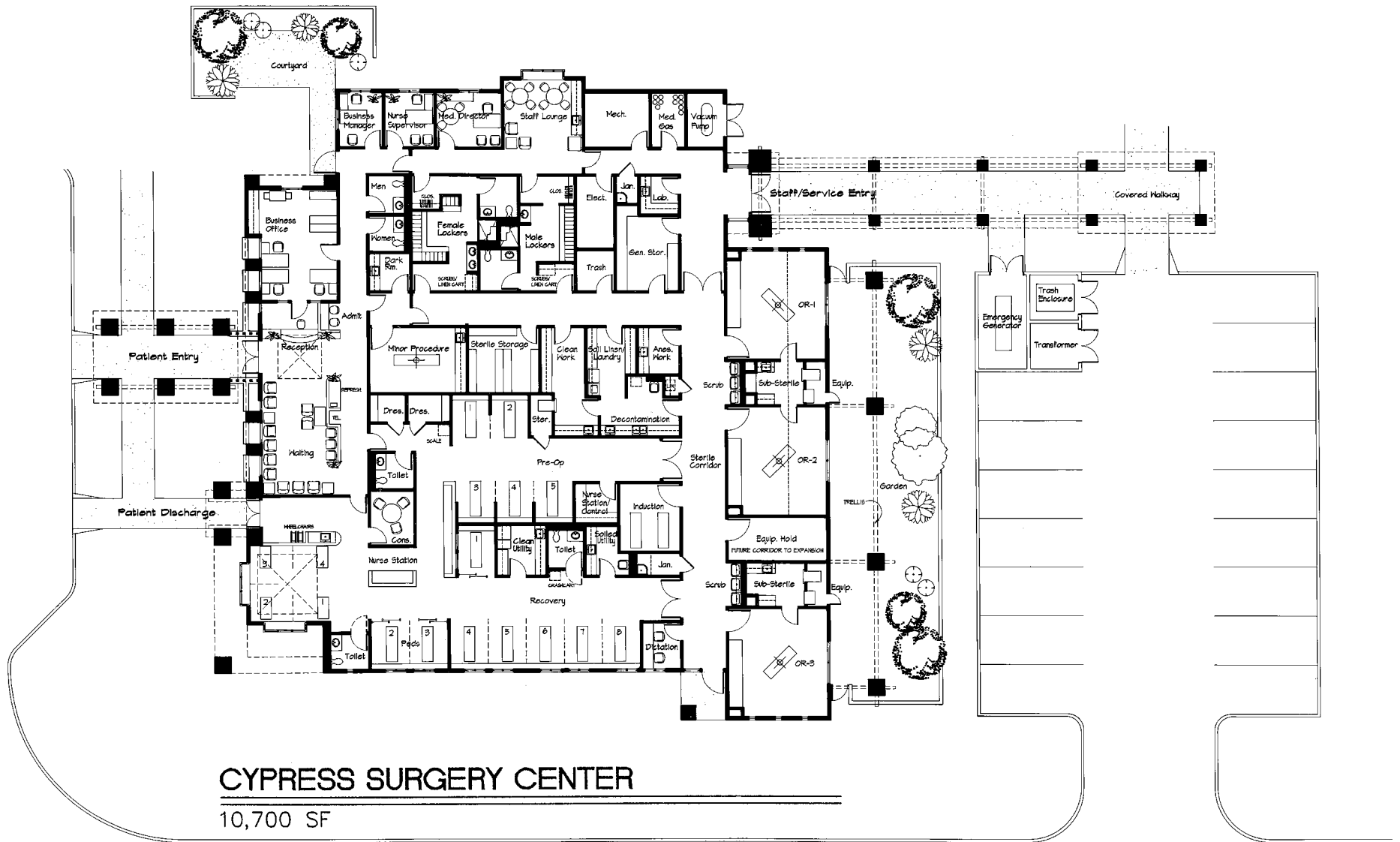
Figure 7-4. Space plan for ambulatory surgical center, 10,700 square feet. (Design: Boulder Associates, Inc., Boulder, CO)
