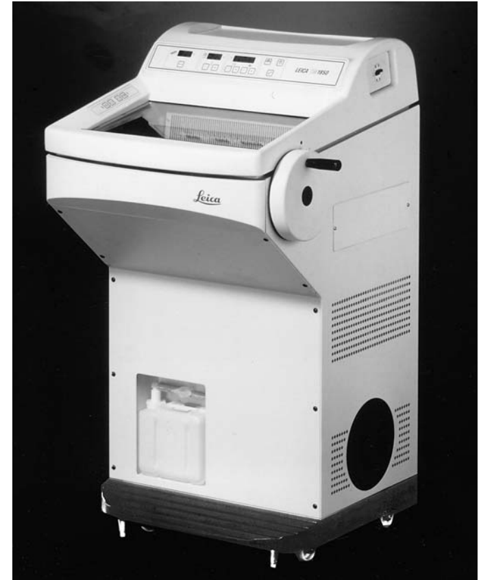
Figure 4-118. Cryostat used for sectioning tissue. Leica CM1900. (Photo courtesy: Leica Microsystems Inc., Bannockburn, IL.)
