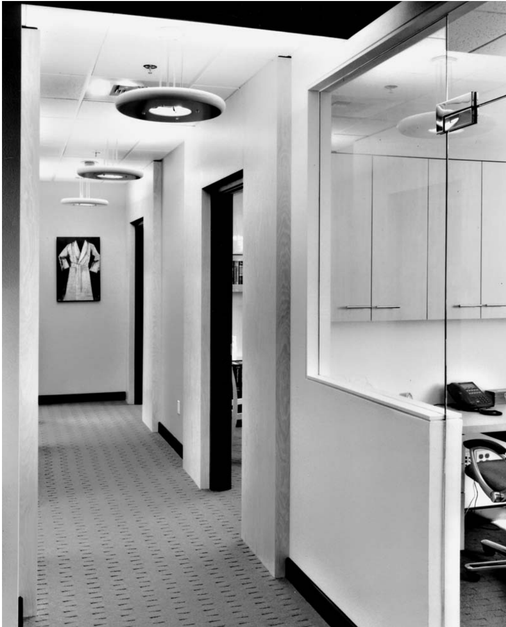
Figure 13-2. Indirect pendant lighting provides soft illumination for corridors. (Design: Jain Malkin Inc.; Photographer: Steve McClelland.)
