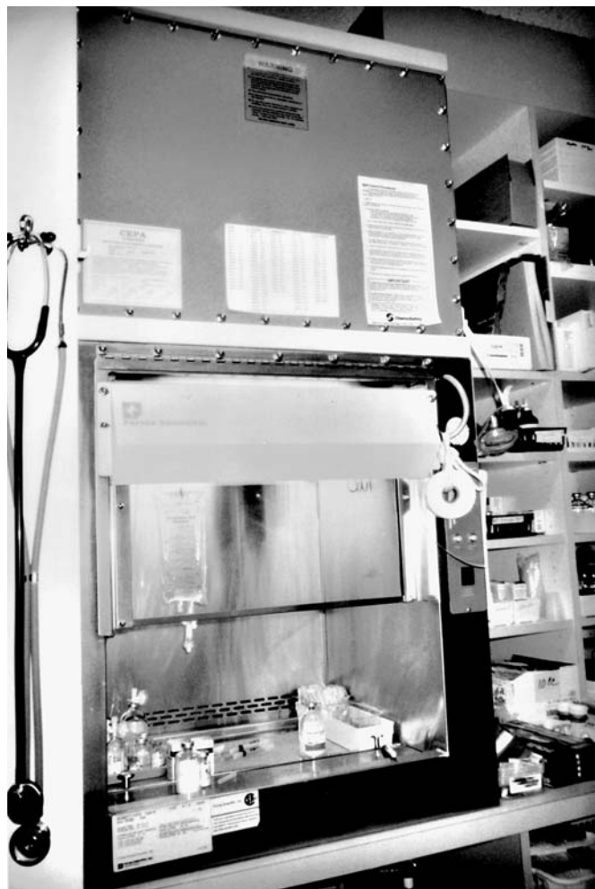
Figure 4-46. Biological safety cabinet used for preparation of chemotherapy drugs. (Photographer: Jain Malkin.)
