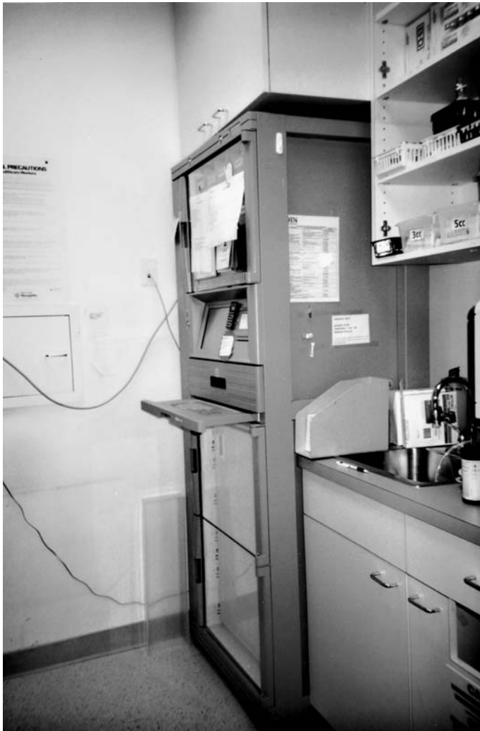
Figure 4-44. Chemotherapy laboratory, oncology suite (wall opposite that depicted in Figure 4-43). Note that the tall cabinet is a refrigerated medication inventory and dispensing unit. (Photographer: Jain Malkin.)
