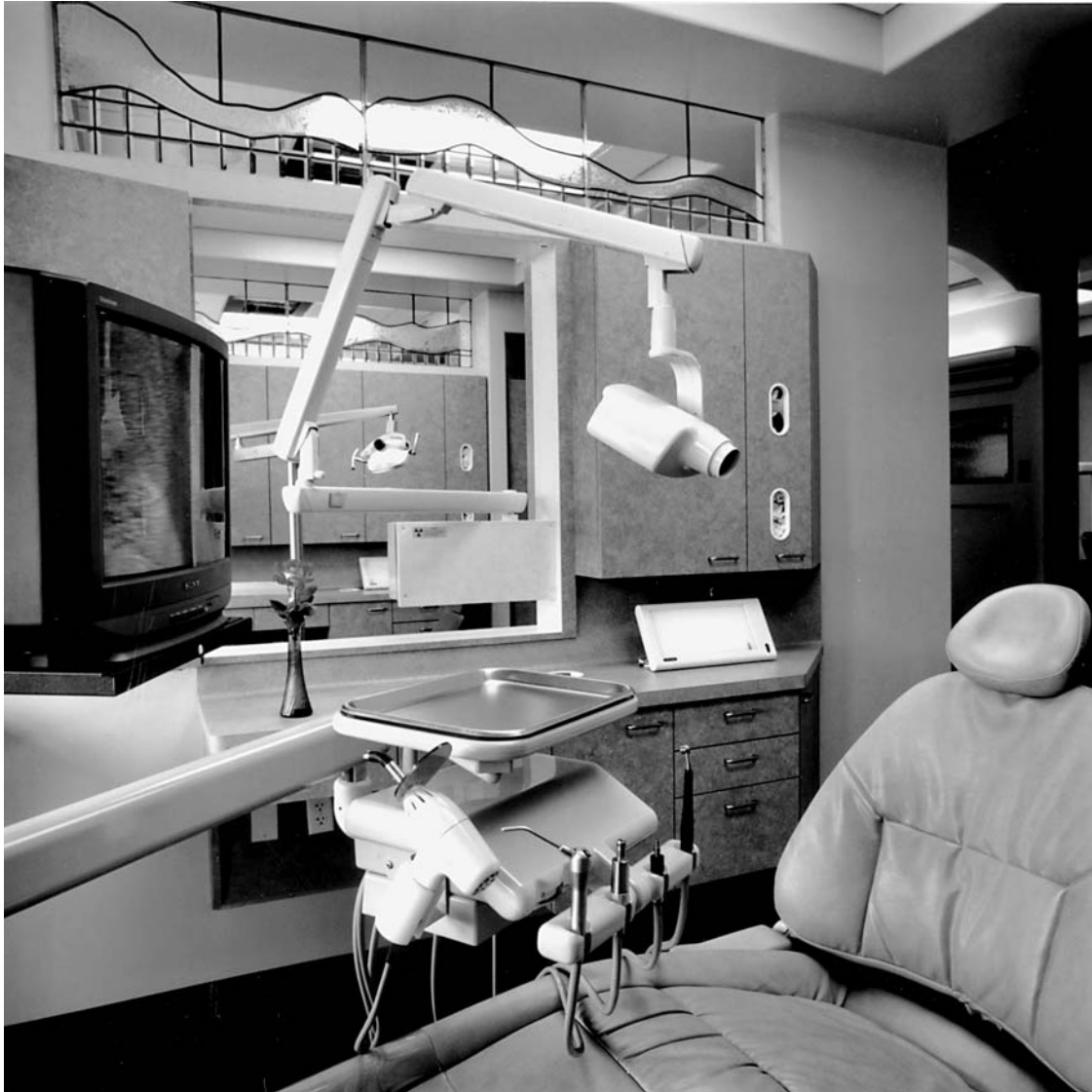
Figure 10-30. Treatment room features wall pass-through intraoral X-ray with leaded art glass above. ( Space planning and interior design: Janet Pettersen, IIDA, Design Wave, Fallbrook, CA; Space planning collaboration and dental equipment engineering: Lee Palmer, Burkhart Dental, San Diego; Photographer: J. T. MacMillan. )
