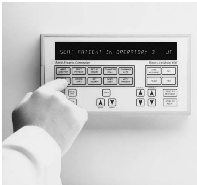
Figure 10-60. Communication system “Direct-Line”™. (Photo courtesy: Amtel Systems Corp., Chester Springs, PA.)
