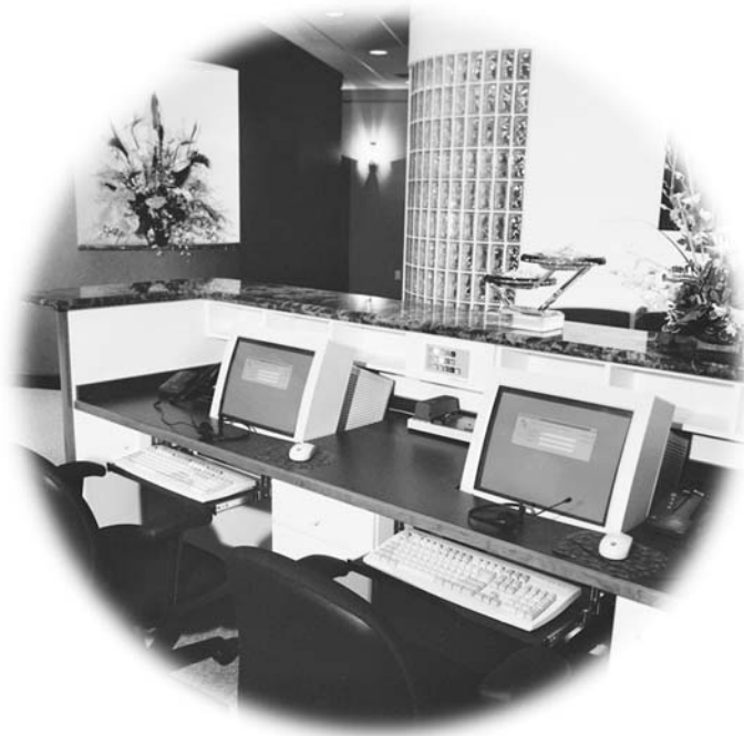
Figure 10-90. Computer monitors recessed into the countertop place screens at proper ergonomic viewing distance and keep them out of the way when greeting patients. (Photo courtesy: Sullivan-Schein Dental, Melville, NY.)
