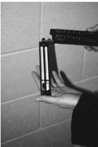
PHOTO 1.1 The thermometers of a sling psychrometer. Note the cloth sock on the wet bulb thermometer. (Used with permission of ABC)
