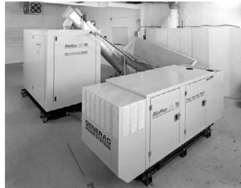
PHOTO 25.14 A small-scale modular biopower system. It is comparable to diesel/gas engine-generator technology except that wood chips are used as fuel. The wood chips are converted to a fuel gas (biomass gasification) and this gas fuels the engine. (Courtesy of DOE/NREL)
