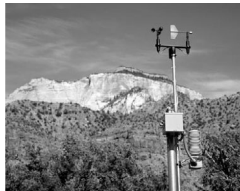
PHOTO 25.28 A cup anemometer (left) and wind vane (right) measures wind speed and direction. (Courtesy of DOE/NREL)
