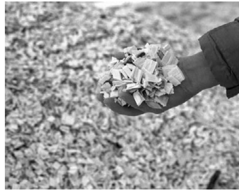
PHOTO 25.13 Wood residues from pulp and paper manufacturing, lumber mills, and other industrial wood users are used for producing biomass electricity. (Courtesy of DOE/NREL)
