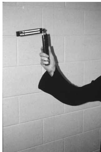
PHOTO 1.2 A sling psychrometer is whirled in the air until the wet bulb temperature and dry bulb temperature achieve equilibrium. (Used with permission of ABC)
