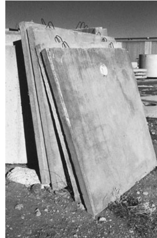
PHOTO 15.4 Concrete baffles used to separate compartments in a septic tank. (Used with permission of ABC)
