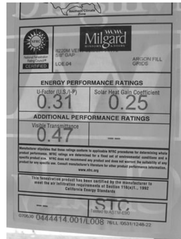
PHOTO 3.13 The NFRC Energy Performance Label that includes ratings of energy performance characteristics on a window. (Used with permission of ABC)
