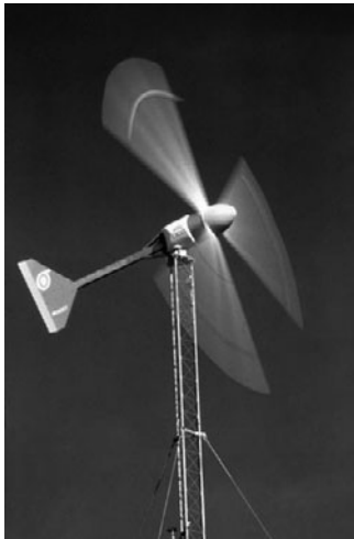
PHOTO 25.30 A Bergey BWC EXCEL 10 kW wind turbine. It is designed to supply most of the electricity for an average total electric home in areas with an average wind speed of 12 mph. (Courtesy of DOE/NREL)
