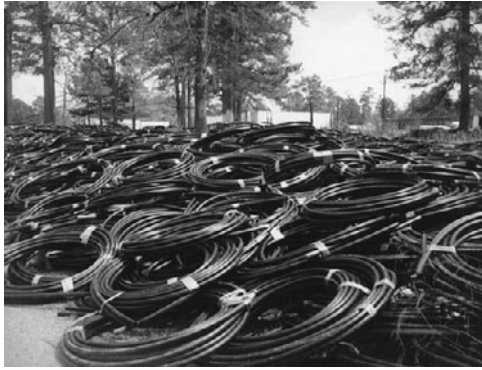
PHOTO 25.7 A 200 ft (61 m) loops as shipped from the manufacturer. (Courtesy of DOE/NREL)
