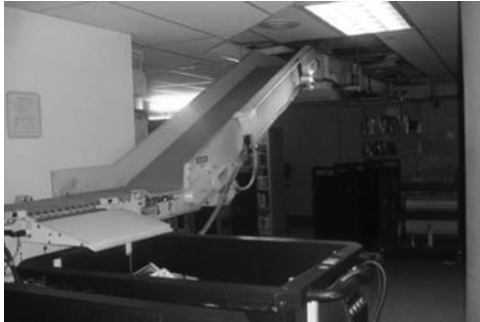
PHOTO 24.16 The conveyor belt of an automatic book-sorting system at a public library. (Used with permission of ABC)
