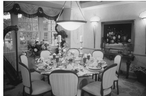
PHOTO 20.28 Ambient lighting provided by decorative ceiling and wall-mounted fixtures. (Used with permission of ABC)
