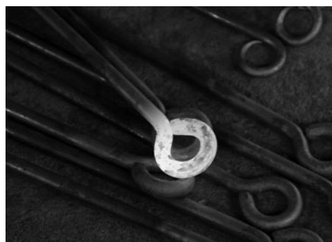
PHOTO 2.1 Glow is the visible part of the thermal radiative energy emitted from the high temperature of the metal object.
