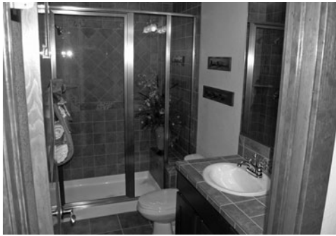
PHOTO 12.21 A three-quarter bathroom (lavatory, water closet, and shower) with glass doors on the shower stall. (Used with permission of ABC)
