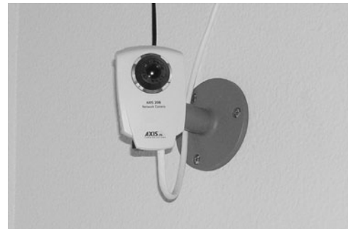
PHOTO 21.29 An indoor camera used for remote surveillance via a local area network or the Internet. (Used with permission of ABC)
