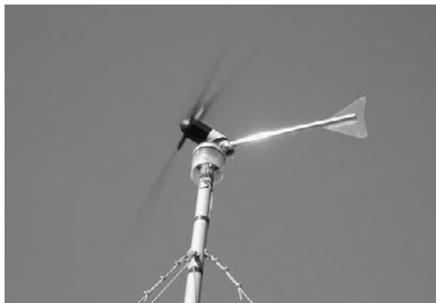
PHOTO 25.31 Furling of the wind turbine to prevent damage in very high winds. (Courtesy of DOE/NREL)
