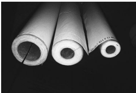
PHOTO 13.27 Pipe insulation with protective sheathing. (Used with permission of ABC)
