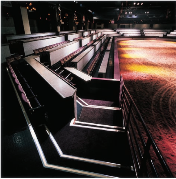
FIGURE 4.13 The Safe-T-First System in light from Johnsonite. The system has won many design awards. It is visible in light and sudden darkness. Photographs courtesy of Johnsonite.
