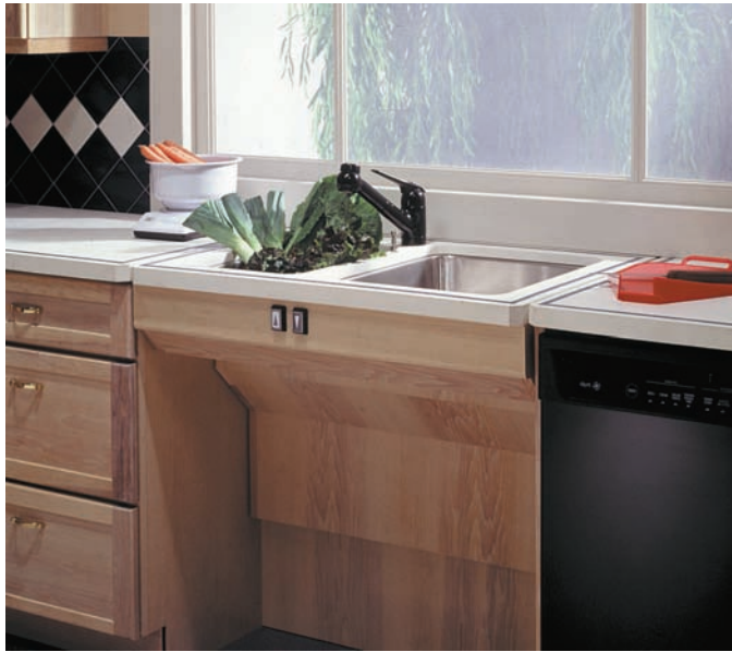
FIGURE 9.2 Approach for the sink. The touch of a button raises and lowers the sink height from 28 to 36 inches. At its lower positions, the height is ideal for seated use or wheelchair heights. Raised to 36 inches, it matches the counter height of standard base cabinets. Photos courtesy of Populus Furniture by AD-AS.
