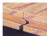
FIGURE 4.4 Solid wood and engineered wood. This illustration not only shows the difference between solid wood and engineered wood but also shows a tongue-in-groove joint. Drawing courtesy of Armstrong World Industries.
