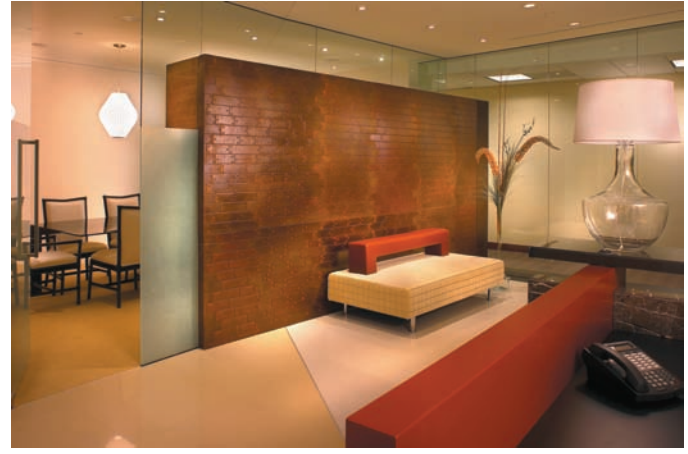
FIGURE 7.3 Over 57,000 pieces of QuarryCast, MetalCast, and Glassfiber Reinforced Gypsum (GRG), representing virtually every column, wall panel, moulding, and so on, are visible in these photographs. Photo courtesy of Formglas.
