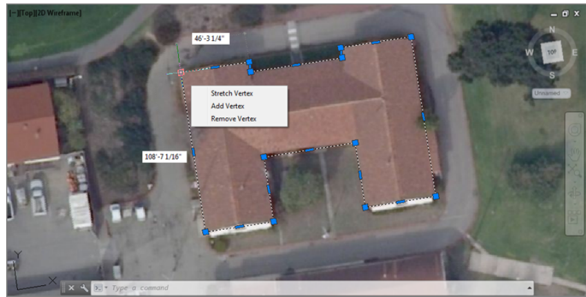
FIGURE 14.21 Dimensions from a building outline
