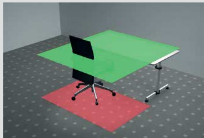
63 Areas defined by DIN 4543: The VDU task area (green) consists of a work surface (white desktop) and a user area (red).
