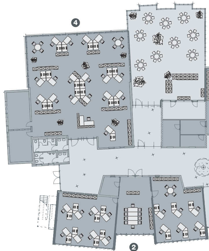
This office building floor plan shows the principal types of office and room, their salient features and the main access zones within the building.
