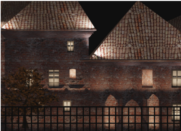
Figure 9: Computer visualization of illumination with the use of metal halide lamps – front view.
