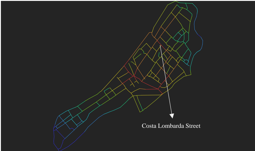
Figure 2: Axial map and an integration value in an old city of Jesi.
