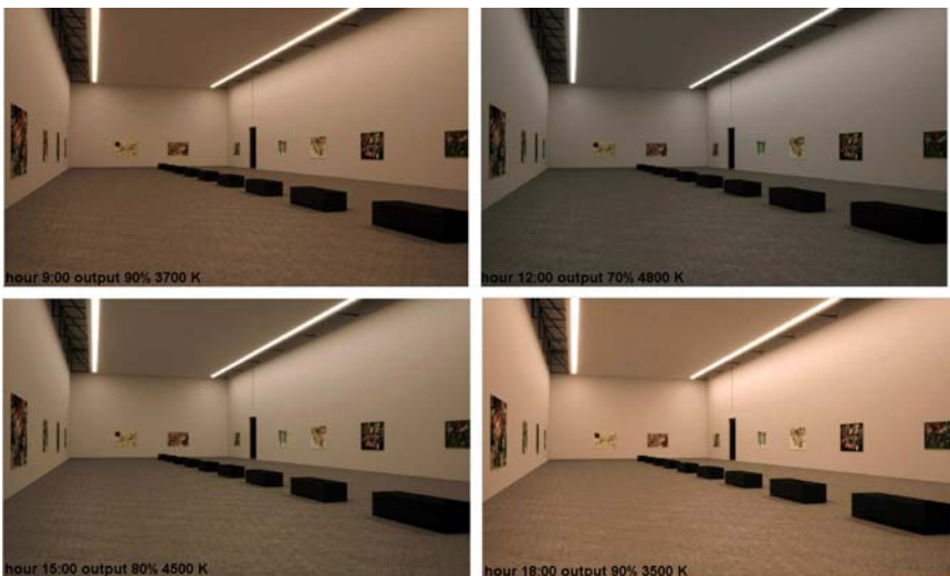
Figure 8: The images of the Exhibition Hall with dynamic lighting system at different hours of the day.
