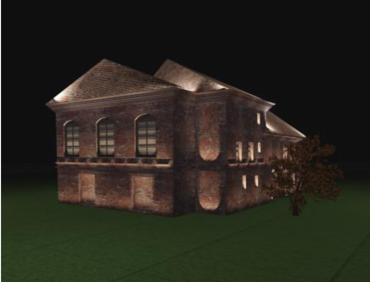
Figure 10: Computer visualization of illumination with the use of metal halide lamps – perspective view.
