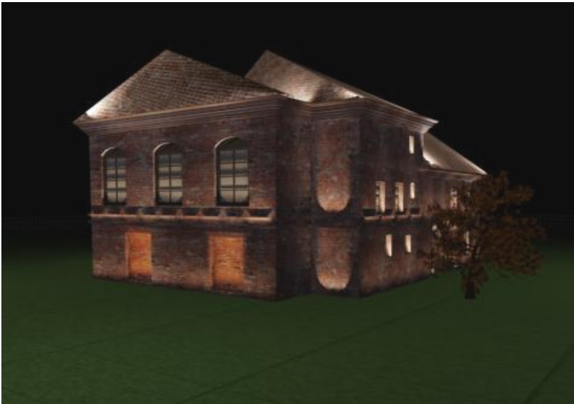
Figure 11: Computer visualization of an object illuminated with metal halide lamps and sodium lamps – perspective view.
