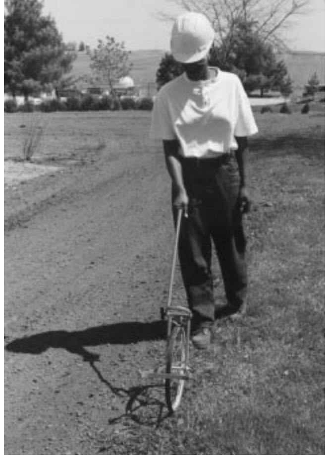
Figure 36-2 Measuring for edging with measuring wheel.
