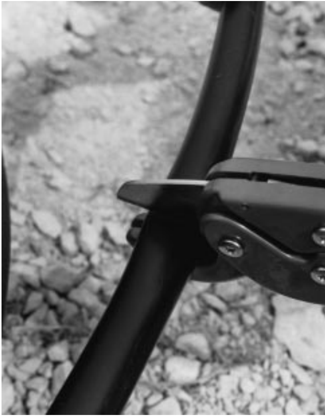
Figure 7-9 Cutting poly pipe using a tubing cutter.
