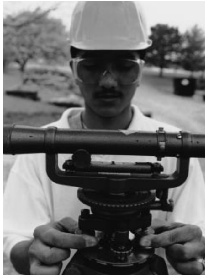
Figure 8-9 Leveling a survey instrument. Always turn the leveling screws in opposite directions.
