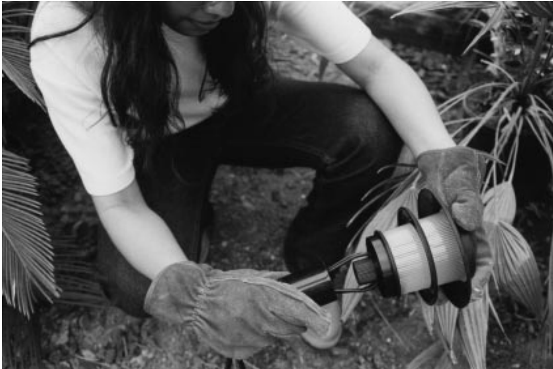
Figure 14-6 Sliding mounting stem over threaded cap.
