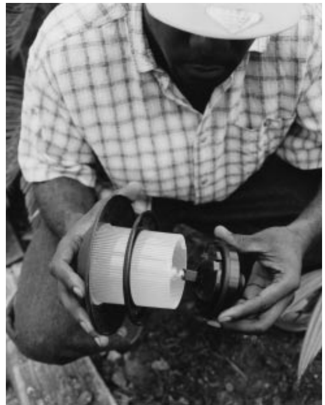
Figure 14-2 Attaching lens to lamp base.
