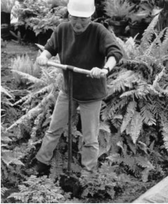
Figure 7-3 Operating auger type posthole excavator.
