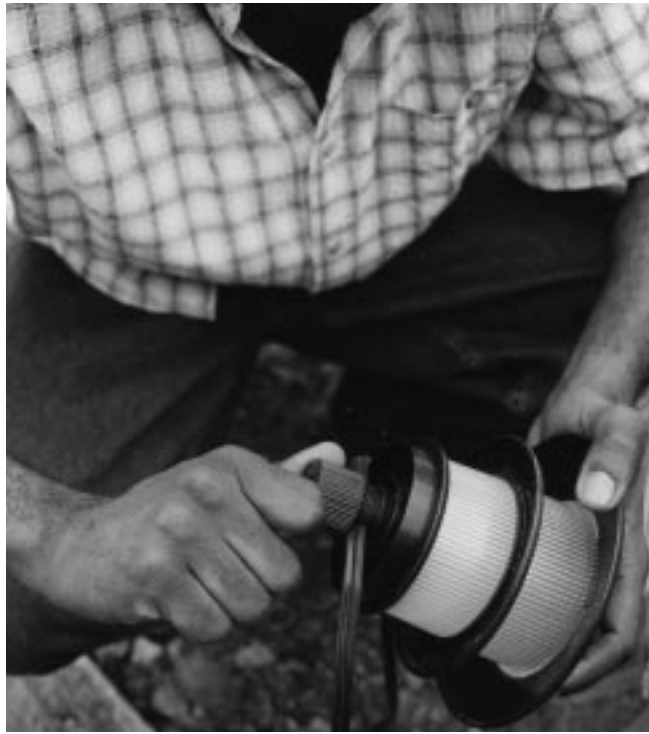
Figure 14-5 Attaching threaded cap to lamp base.
