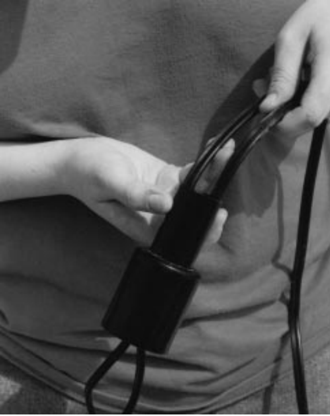
Figure 14-3 Running loop of cable through mounting stem.
