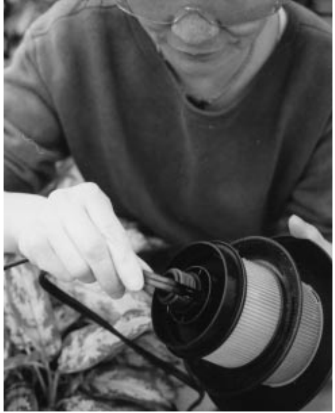
Figure 14-4 Connecting cable to lamp base. A metal prong must penetrate each side of the cable for the light to work. Do not bend the metal prongs.
