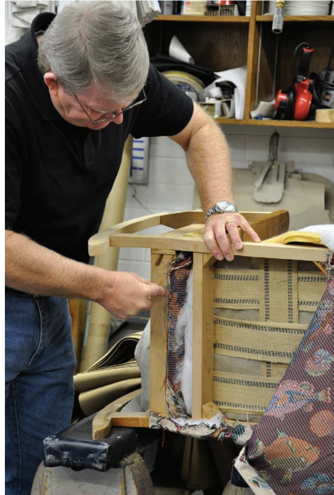
Figure 9.6 An upholsterer removes the worn fabric of this chair to begin the process of reupholstery. Revealed is the webbing on the back, padding and batting of the arm, and the frame of the piece. Photo © Kathryn Taylor
