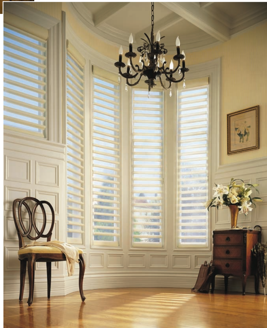
Figure 11.21 Pirouette® window shadings appear as soft shutters. These have an ingenious construction—a double layer of sheer polyester fabric with fused opaque fabric slats between that are adjustable from fully open, as seen here, to completely closed for privacy and light control. These shadings roll up into the headrail to fully expose the glass. This treatment assures both day and nighttime privacy and are excellent as stand-alone window coverings or for the privacy and glare control layer beneath decorative fabric treatments. Photo courtesy of Hunter Douglas
