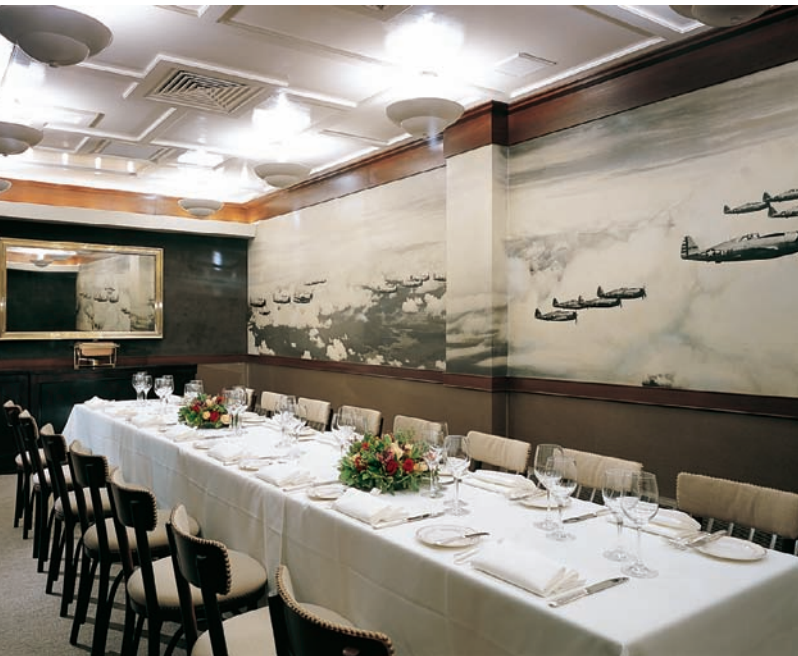
Figure 2.7 Energy-saving compact fluorescent lamps create ambient light in this restaurant. © Peter Mauss/Esto
