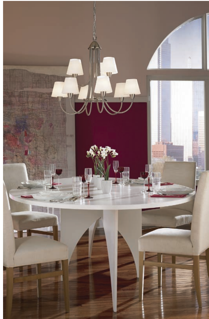
Figure 5.1 The contemporary chandelier in this dining space is well placed to be about 36 inches above the table. The suspended light balances natural light from the right, making the space practical and psychologically pleasing. Photo courtesy of Sea Gull Lighting Products, LLC
