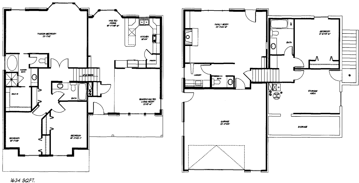
Figure 7.8 A split-level home showing three steps down to the family room and ten steps up to the bedroom wing above the garage. Storage and one more bedroom are beneath the kitchen and living room. CAD by Gary Stewart
