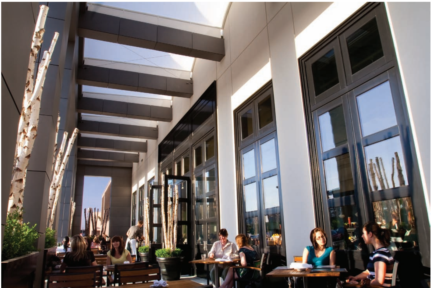
Figure 1.2 Interior design can be observed and evaluated in places where we shop, worship, do business, or obtain services such as dining in restaurants. At the Oliver and Bonacini Café & Grill, a contemporary patio space has been added to the existing structure where natural lighting is enjoyed through retractable textile membrane vaults overhead and through commercial French doors. Furniture placement allows many diners to enjoy this sunny space, accessorized with tree trunks and large planters of greenery. Design by Anacleto Design Associates/photo courtesy of Eventscape, Inc.
