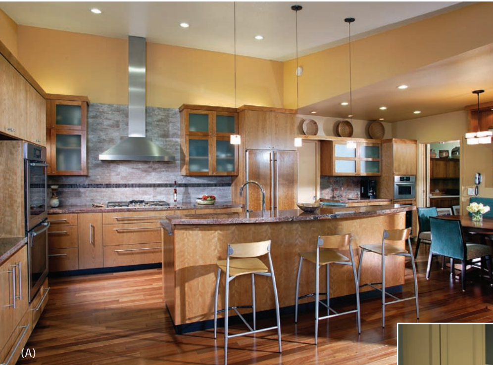
Figure 6.16 Two well-planned kitchens. (A) This Modern kitchen features a cooktop, or range, in the center of the longest wall with plenty of countertop for food preparation on each side. Double wall ovens to the left aid in baking efficiently. The island features the sink/cleanup zone, allowing a view to the great room while at work. Bar stools show informal dining, with the dining table with pendant lighting and a dinnerware storage hutch to the right. (B) This HGTV Dream House kitchen in Farm Country style also features a central cook space, this one with a large gas cook surface and double lower ovens and space to each side. Double refrigerators flank the preparation area and a pantry at the right gives ample space for food and a butler's pantry for serving items. The sink is in the center of a large food preparation and serving island with dining table nearby. (A) Design by Gioi Tran, Co-Designers: Meghan Nohr; Applegate Tran Interiors/Photography: Dave Adams/NKBA Design Competition; (B) photo courtesy of HGTV
