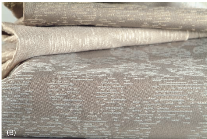
Figure 2.5 (A) Xorel® is a sustainable fabric made of polyethylene (PET)—produced without the use of plasticizers, chlorine, or PVC. Once installed, Xorel® offers extremely low toxicity and off-gassing, making it a clean-air choice, as well. (B) Insight® is made of polylactic acid, derived from corn syrup, a renewable resource from which this sustainable, green-design fabric is produced. It is completely biodegradable. Photos courtesy of Carnegie Fabrics: www.carnegiefabrics.com
