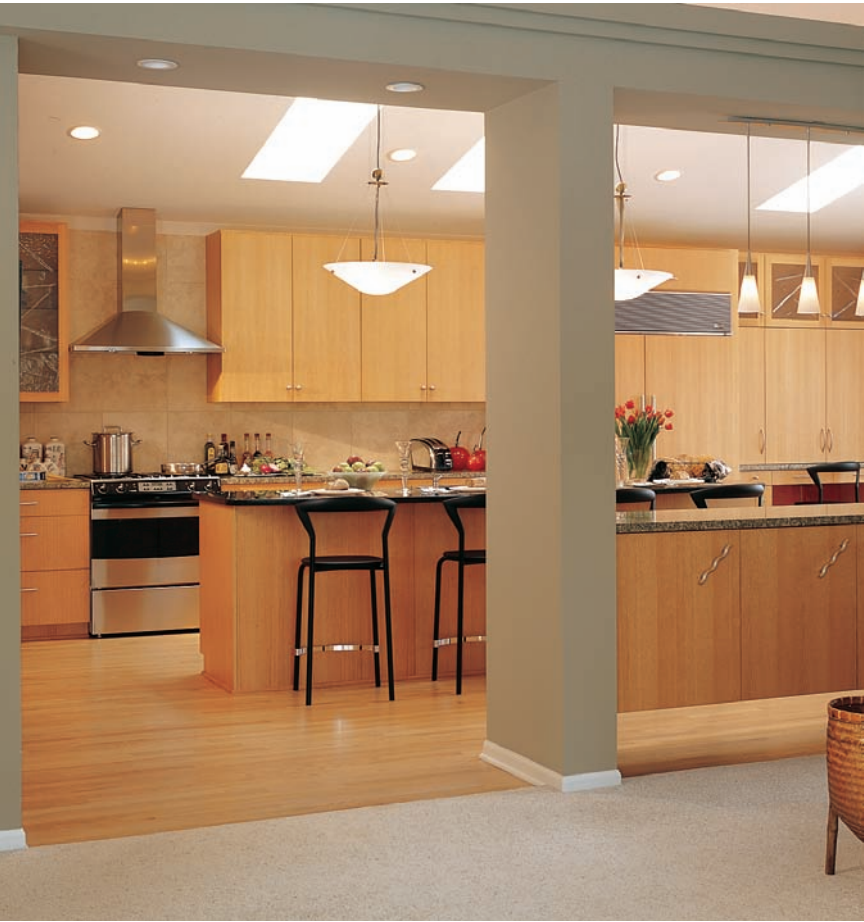
Figure 5.18 Architectural lighting is seen in this well-lit kitchen as luminous panels for general lighting with supplemental downlights. Suspended luminaires include a pair of pendant fixtures and a trio of minipendants. © Susan Gilmore/Esto
