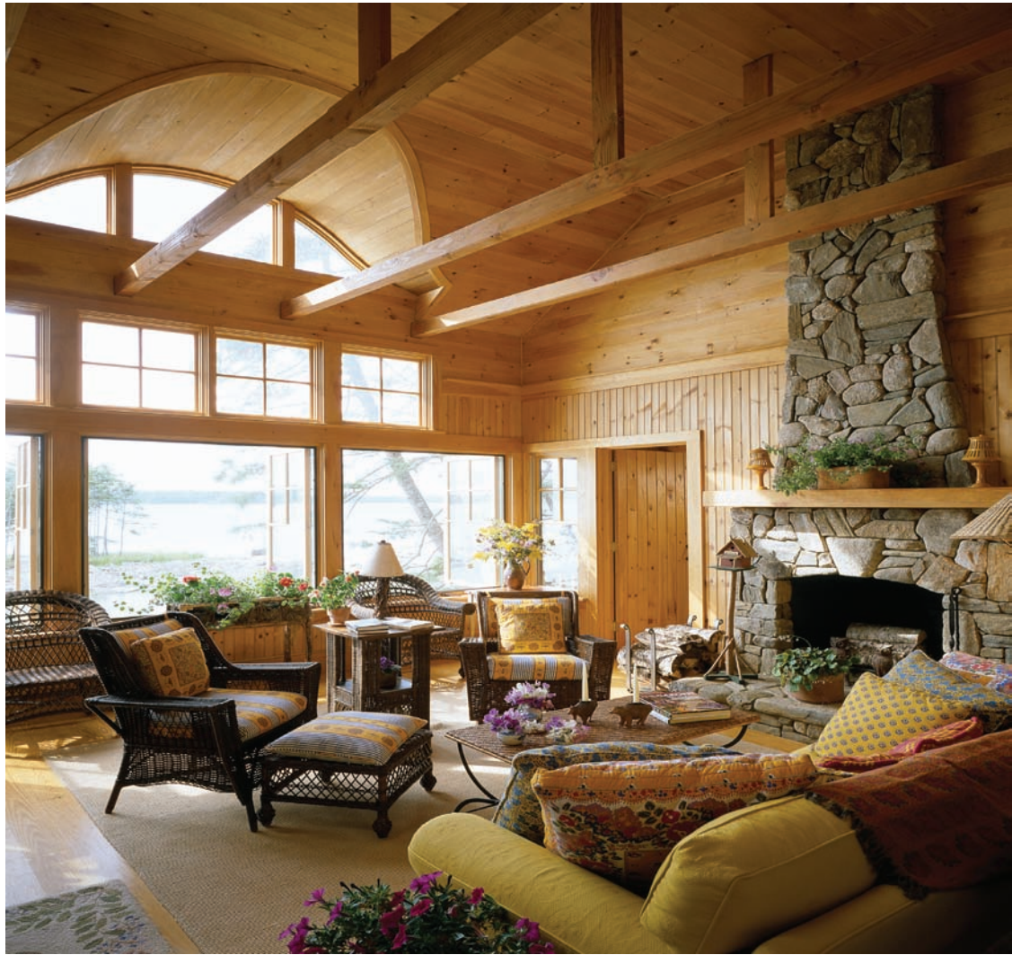
Figure 10.34 A richly architectural interior, this room features case-ment windows with four-pane transom or clerestory windows above and crowned with an arched window. Beams, wood paneling, and a stone fireplace are all tactile, handsome elements. Design by Bernhard & Priestley Architects/photo © Brian Vanden Brink
