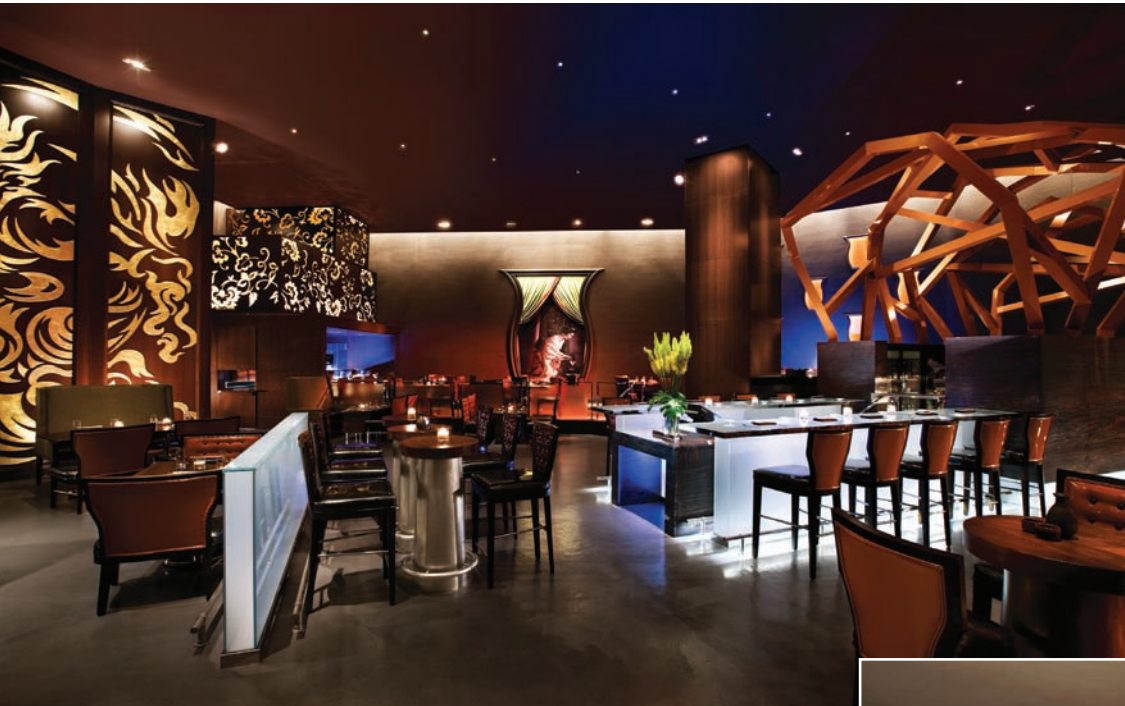
Figure 5.16 The Izakaya Restaurant in Atlantic City, NJ, is filled with mood-manipulating lighting. Effects include direct downlighting over dining tables, ambient/accent lighting on large-scale Japanese patterned screens, accent highlighting of the impressive custom structure that defines the entryway, and fluorescent lighting that draws attention to the central counter dining. The combination of lighting effects creates a place for elegant, ritualistic dining in an unhurried, elegant atmosphere. Design by Alvarez-Brock Design/photo courtesy of Eventscape, Inc. www.eventscape.net
