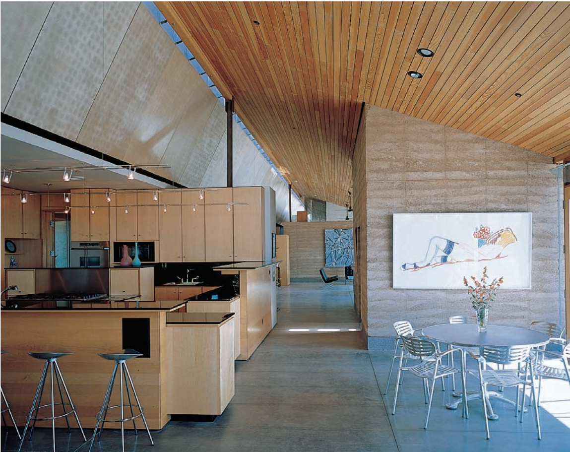
Figure 7.26 This Arizona home receives abundant natural light through a long, narrow north-facing skylight and expanses of south-facing glass. Direct solar gain from the south is permitted in winter and obstructed in summer by a deep, precisely angled roof overhang. A high-efficiency heat pump fulfills all heating and cooling functions. Eddie Jones Architect, Phoenix. Photo © Timothy Hursley/The Arkansas Office, Inc.
