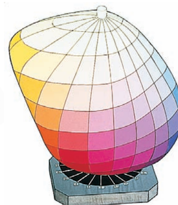
Figure 4.9 The Munsell color notation system in three-dimensional form. Courtesy of Gretag/Macbeth, New Windsor, NY
