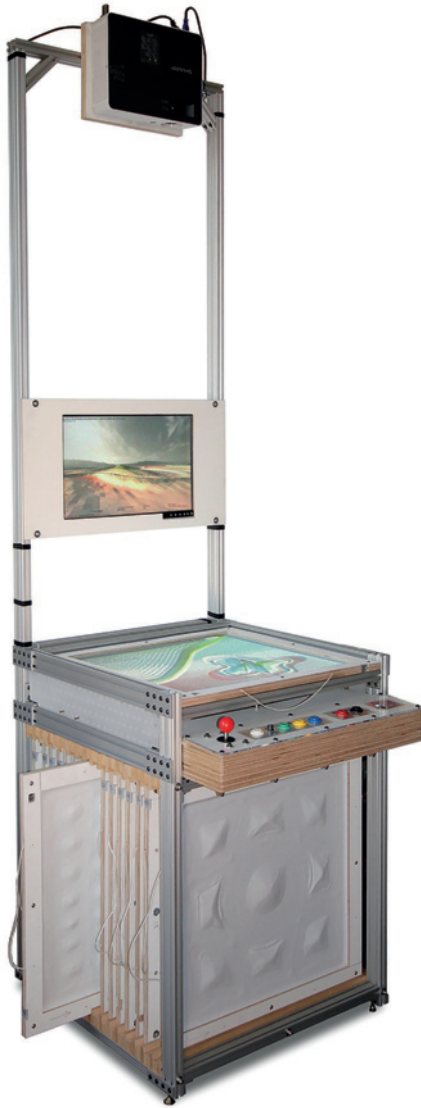
Figure 2.4 'Greetings from the Owens Lake' public interface system with 17 vacuum-formed sand-modeled dust control landscapes, arcade-style controls, first-person display and overhead projection, and embedded postcard printer.
