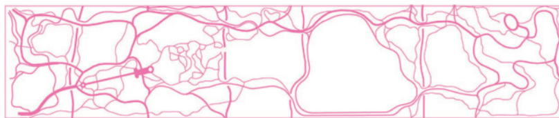
Figure 12.9 Site plan – Central Park, New York City, circa 1875. The park's network of paths is split into visitor passages and service roads; while they may appear to be organic, the landscape architect, Frederick Law Olmstead, carefully planned for their separation.
