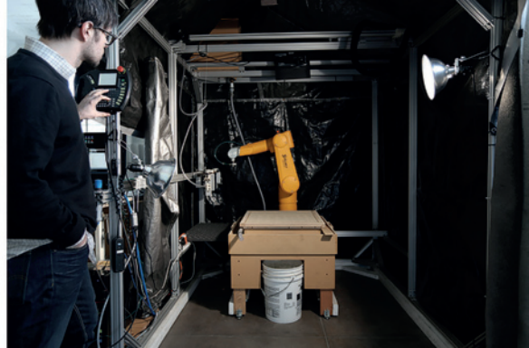
Figure 2.3 Rapid Landscape Prototyping Machine topographic sand modeling system with robotic arm, 3D laser scanner, vacuum-forming sandbox, and digital projection system.
