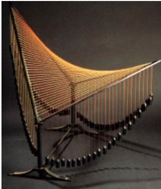
Figure 4. Model of hyperbolic paraboloid A parametrically variable analogue model of a hyperbolic paraboloid.
