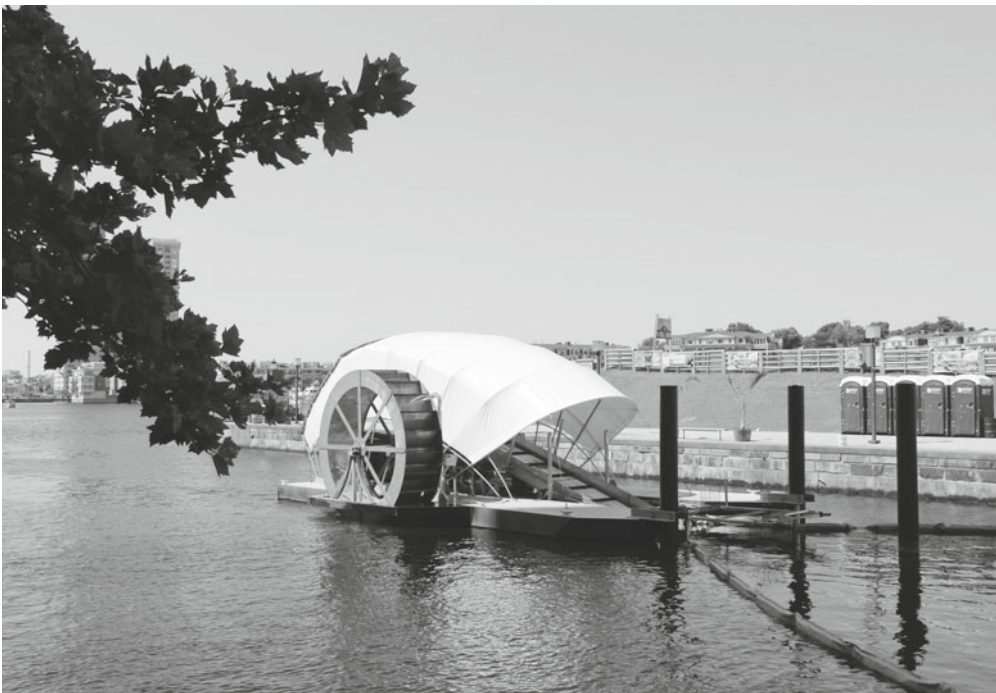
This unusual solar- and water-powered water wheel collects garbage before it enters the inner harbor of Baltimore, Maryland. Photo Credit: Baltimore Healthy Harbor Initiative.
