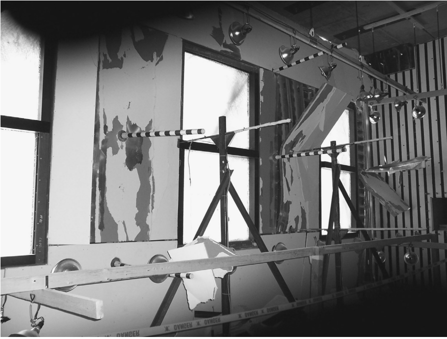
Figure 5.4 Digital Photography and Deflection Measurement
