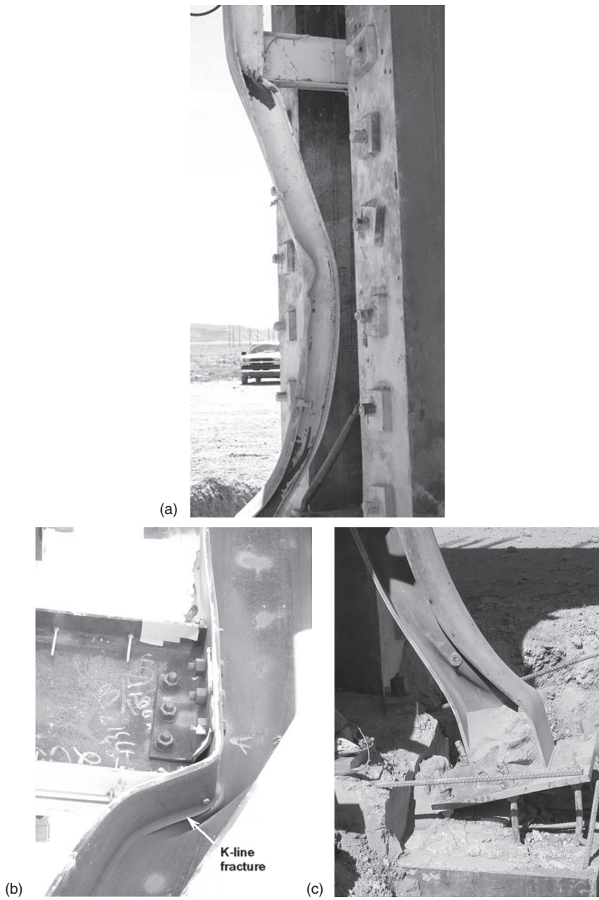
Figure 17.7 Examples of failure modes for steel columns: (a) Section view, illustrating Mode 1 P- \delta failure, (b) Connection view, illustrating concerns with fracture (Mode 3 failure), (c) Baseplate view, depicting a Mode 2 failure (Photo courtesy of DTRA)
