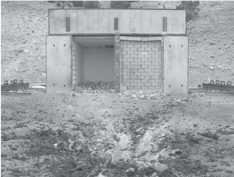
Figure 17.9 Example showing the benefit of using FRP to retrofit a masonry wall to enhance its blast resistance: (a) Control (left) and retrofitted wall (right) prior to blast test, (b) Control (left) and retrofitted wall (right) after the test (Photo courtesy of The Energetic Materials and Research Testing Center)
