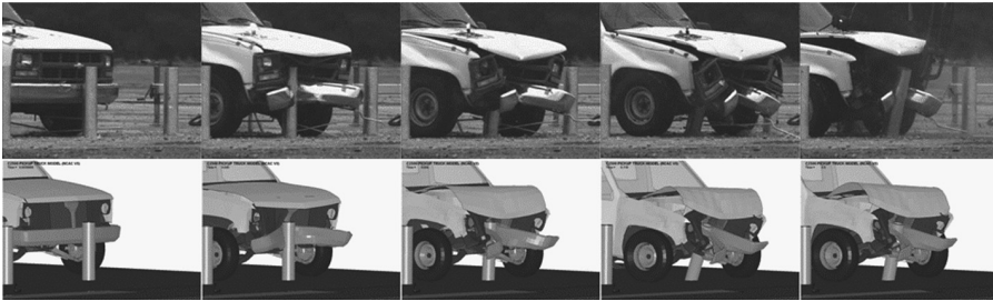
Figure 12.6 Comparison of Vehicle Impact Test to Finite Element Analysis (Compliments of Applied Research Associates, Inc.)
