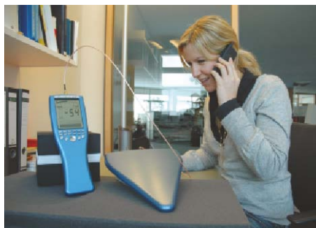
Fig. D9.4 Workstation EMC measurement
