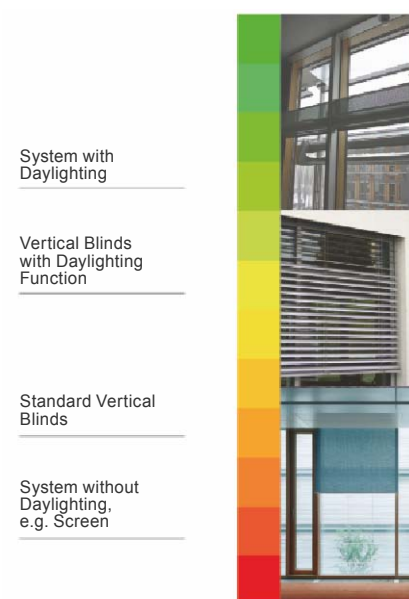
Fig. C1.42 Classification of solar protective systems in regard to the level of existing daylighting
