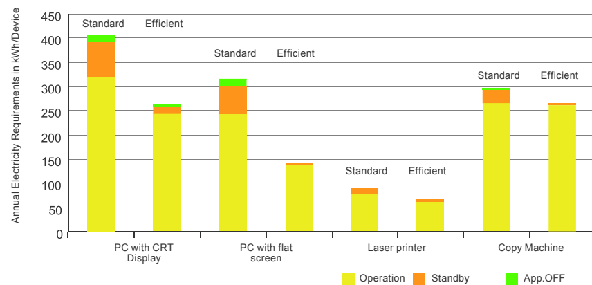
Fig. B2.22 Electricity Demand for work aids. Through the use of energy-efficient appliances, electricity demand can be decreased by up to 50% when compared with standard appliances.
