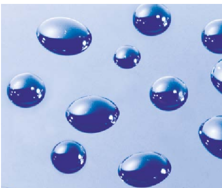
Fig. C1.65 Self-cleaning glass coating with silicon-chemical compounds that allow for water to drip off easily
