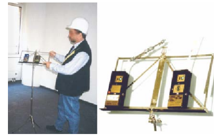
Fig. C3.7 Measuring air quality after building takeover
