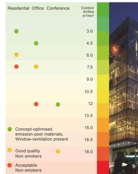
Fig. B1.43 Hygienically required surface-related outdoor airflow rates for different utilizations
