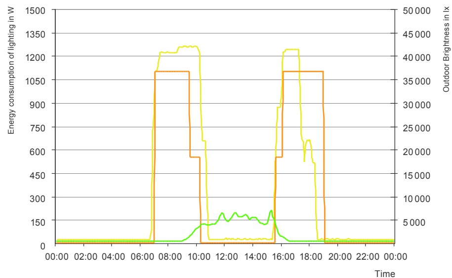
Fig. D4.3 Electricity consumption for lighting for a communal office
