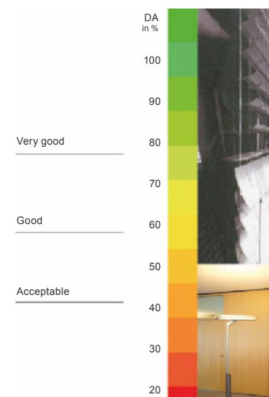
Fig. B2.14 Parameters for daylight autonomy (DA) for a typical office in Central Europe
