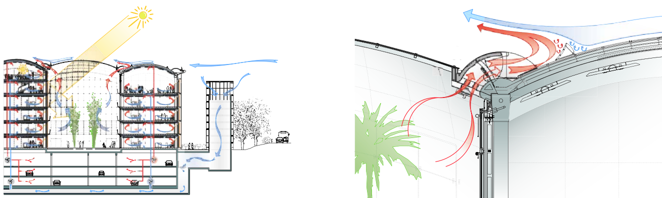
Fig. C1.48 Natural ventilation concept for atria in the Lufthansa Aviation Centre/Frankfurt in Germany. Architects: Ingenhoven Architekten, Duesseldorf
