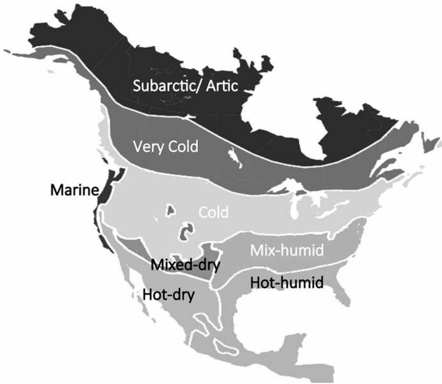
FIGURE 3.12. EEBA Climate zone map. Credit: Adapted from Energy and Environmental Building Association.
