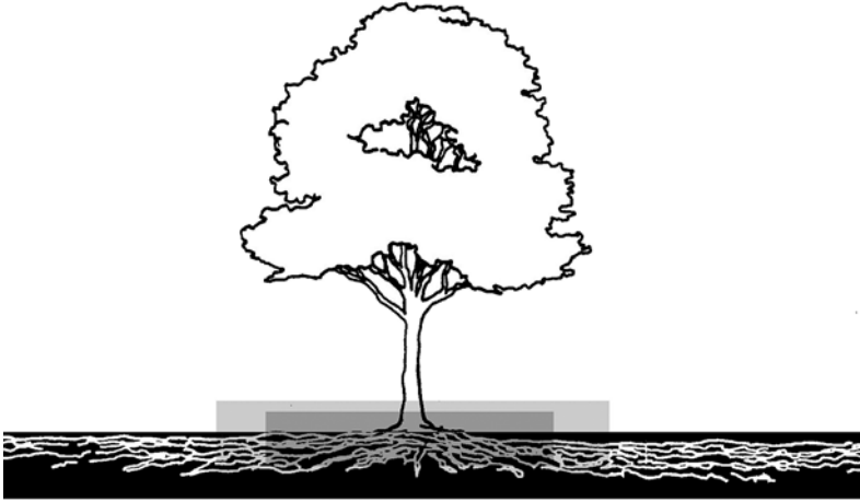
FIGURE 5.2. Tree root zone protection should be placed out to the drip line.
