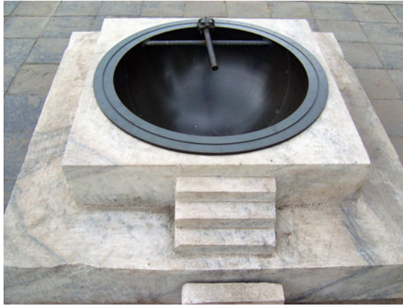
Fig. 2.37 This Scaphe is a one-fourth-scale replica of the original created by Guo Shoujing (1231–1316). It is actually a spherical sundial composed of an upward-looking cauldron, two crosses, and a silhouette aspheric board. The device was used to determine the sun’s spherical location; it could also be used to measure solar displacement throughout the year and observe solar eclipses. Source Photograph by Changsong Wang
