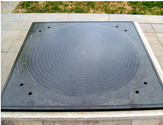
Fig. 2.36 The Direction Determining Board is a device used for establishing directional orientation. Invented by Guo Shoujing (1231–1316), the device was originally of wooden construction, but in later times copper was used instead. The square board measures four chi to a side. Source Photograph by Changsong Wang. Note Chi, cun and zhang are traditional Ancient Chinese units of length. 1\text{ m} \approx 3\text{ chi} , 1\text{ m} \approx 0.3\text{ zhang} , 3.33\text{ cm} \approx 1\text{ cun} .
