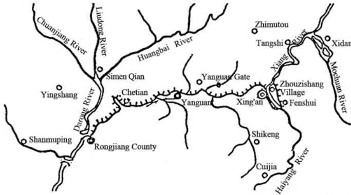
Fig. 8.41 Diagram of the Lingqu Canal. The Lingqu Canal is located in Xing’an County in northern Guangxi Province. The county sits along the Hunan–Guangxi Corridor, which runs from northeast to southwest. The canal, which connects the Xiang and Li Rivers, is 34 km in length. Source Editorial Committee on the Lingqu Canal in Xing’an, Guangxi Institute of Education 1974: 2
