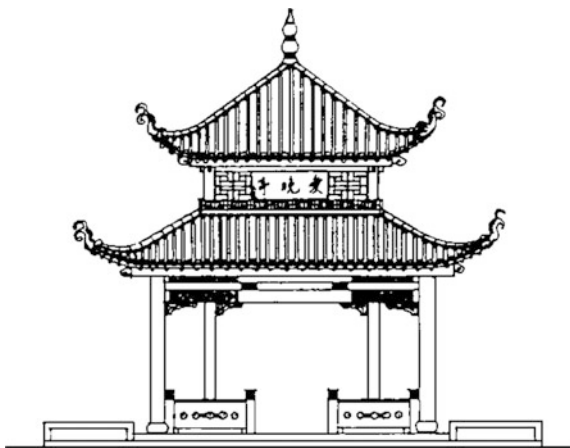
Fig. 5.6 The elevation of the Love Nightfall Pavilion. The pavilion is a classic example of ancient pavilion architecture. The structure has a square base that measures 6.23 m on each side and is 12 m tall. The roof is two-layer double-eaved and has upturned eaves. Source Yang (1993: 206)
