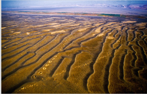
Fig. 8.53 The Gobi desert is one of the most distinctive natural landscapes of the Turpan-Hami Basin. The Turpan Karez System forms a unique scene amidst this dry landscape because of the perfectly aligned vertical shafts. Source Photograph by Bin Huang
