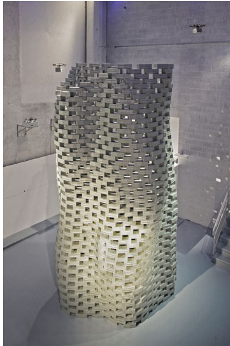
Fig. 2 Flight Assembled Architecture represents the first architectural installation assembled by flying robots and was demonstrated in 2011 at the FRAC Centre, Orléans, France (Image by François Lauginie)
