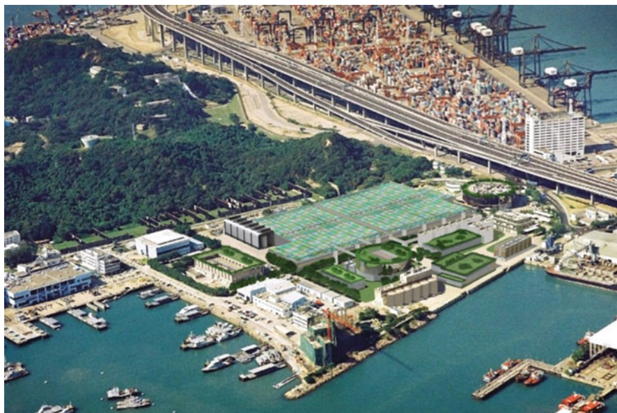
Fig. 4 Upgrading work at Stonecutters Island Sewage Treatment Plant under HATS Stage 2A increases its chemically enhanced primary treating capacity from 1.7 million m 3 to 2.45 million m 3 , serving 5.7 million people (DSD 2010) (©Arup)
