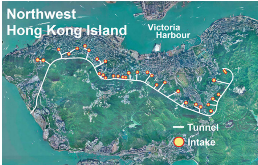
Fig. 9 West Drainage Tunnel is about 10.5 km long, diameter from 6.25 m to 7.25 m with 34 intakes and a total of about 8-km adits connecting the intakes with the drainage tunnel (©Arup)
