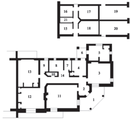
Figure 2.24 “Plan of junior houses in Braim, Abadan,” 1943. 1) terrace; 2) foyer; 3) dining room; 4) pantry; 5) kitchen; 6) backdoor entrance area; 7) toilet; 8) bath; 9) closet; 10) closet; 11) living room; 12) bedroom; 13) bedroom; 14) corridor; 15) storage flanked by toilet; 16) storage flanked by toilet 17) “boy room”; 18) “boy room”; 19) garage; 20) garage. Courtesy of the archives of the oil headquarters in Abadan, Iran. Plans reproduced by Parham Karimi
