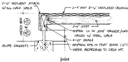
**joist anchor** A metal tie for anchoring joists to a wall or larger structural member.
