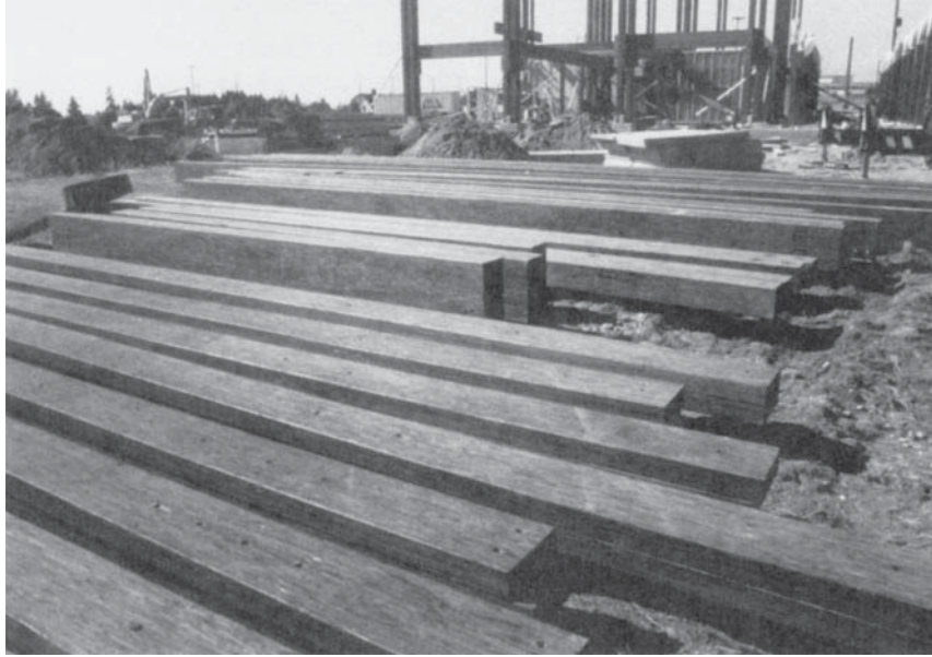
Figure 6.31a Parallel strand lumber. (Photo courtesy of Trus Joist—A Weyerhaeuser Company.)
