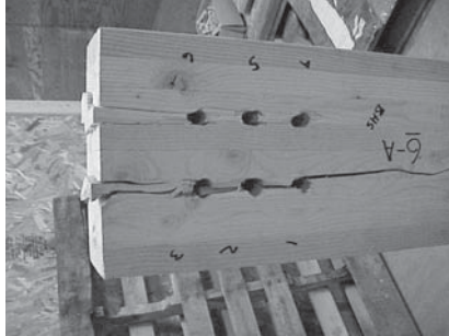
Figure 13.13 Row tear-out failure in the main member for a multiple-bolt connection. Shear plug failures occur between the last bolt in a row and the end of the glulam member.
