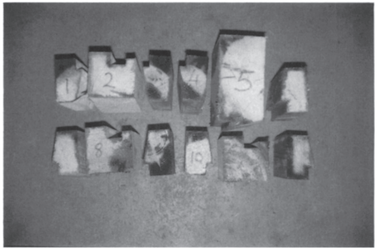
Plate 26. Penetration of wood preservative. Penetration depends on the properties of the preservative and the wood, as well as the moisture content of the wood; in sample 1 the sapwood is completely penetrated, but in sample 11 sapstain deterioration has increased porosity and allowed some penetration into the heartwood, whilst only limited penetration has been achieved in sample 2 because it had a high moisture content and no space for the preservative.
