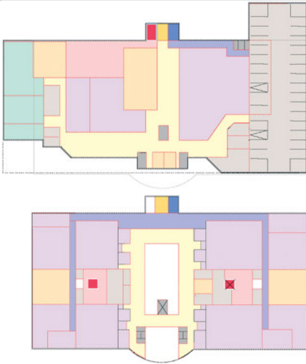
Two floors of a test building model for early concept design. The models consist of 3-D departmental-level spaces laid out on floor slabs without interior separating walls, but with exterior walls for each floor level.
