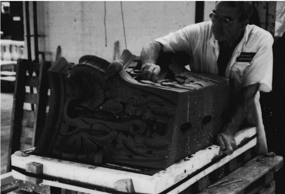
Fig. 3.20 Hand finishing a decorative terracotta block at Ibstock Hathernware Limited, Leicestershire.
