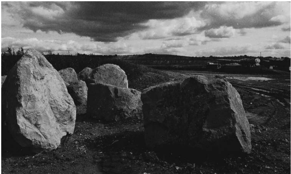
Fig. 3.16 Clunch, a compacted type of chalk from the Cretaceous formation in East Anglia, being quarried at Barrington, Cambridgeshire.
