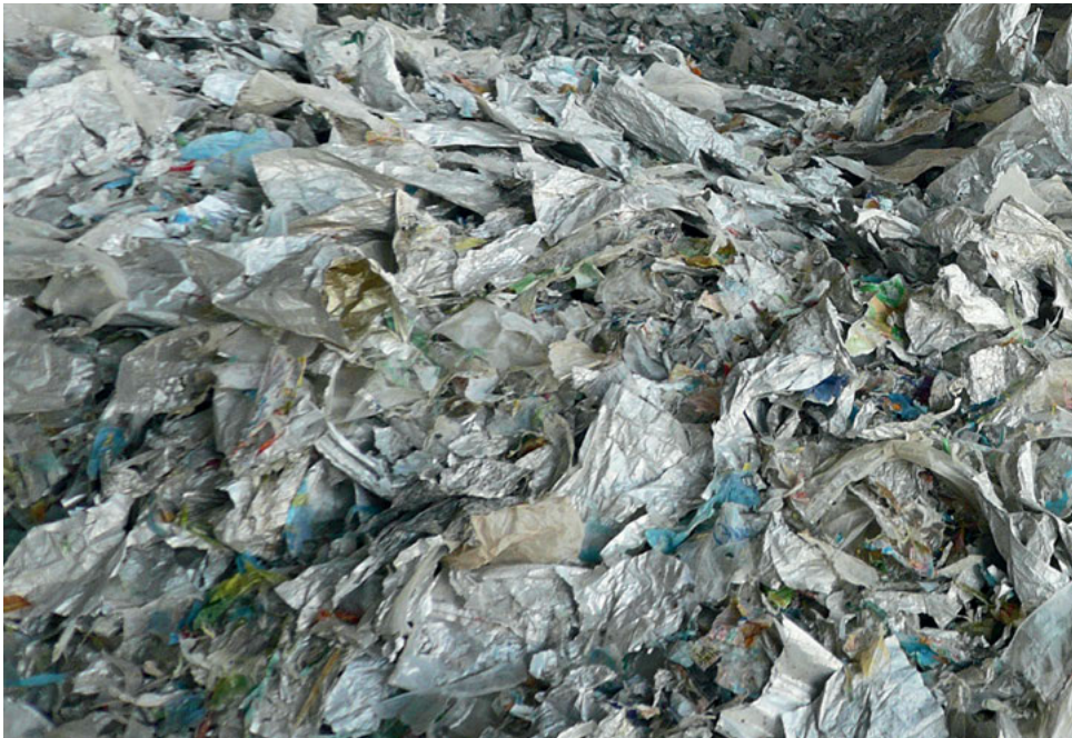
1 Layers of aluminium, paper, and plastic provide the resource for alternative roofing sheets made out of discarded Tetra Pak cartons.
