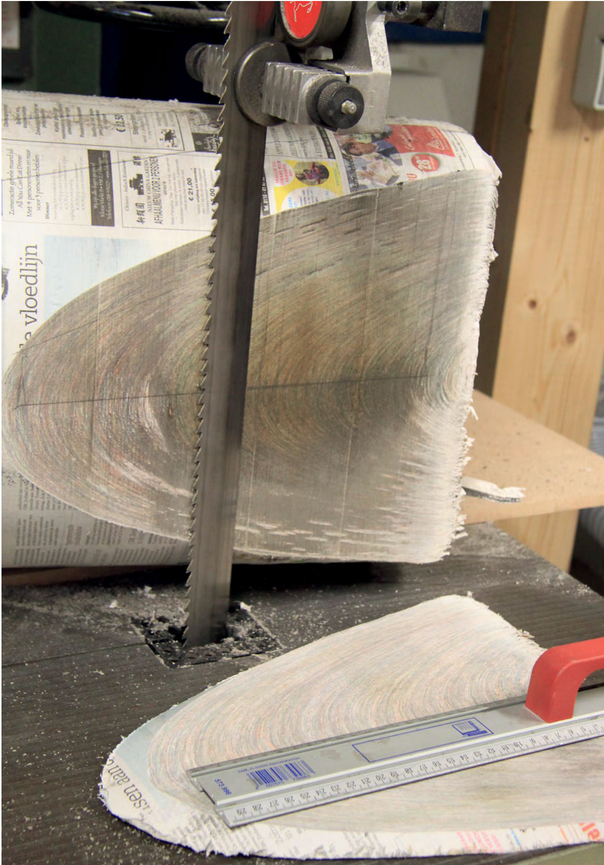
4 Newspaper sheets are rolled up and glued together, forming a log, then cut into any desired shape.
