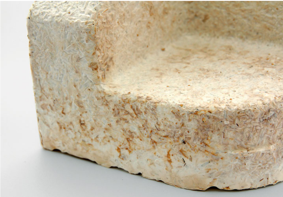
2 Mushroom mycelium can be cultivated to grow into any desired form, here as specially shaped packaging material.
