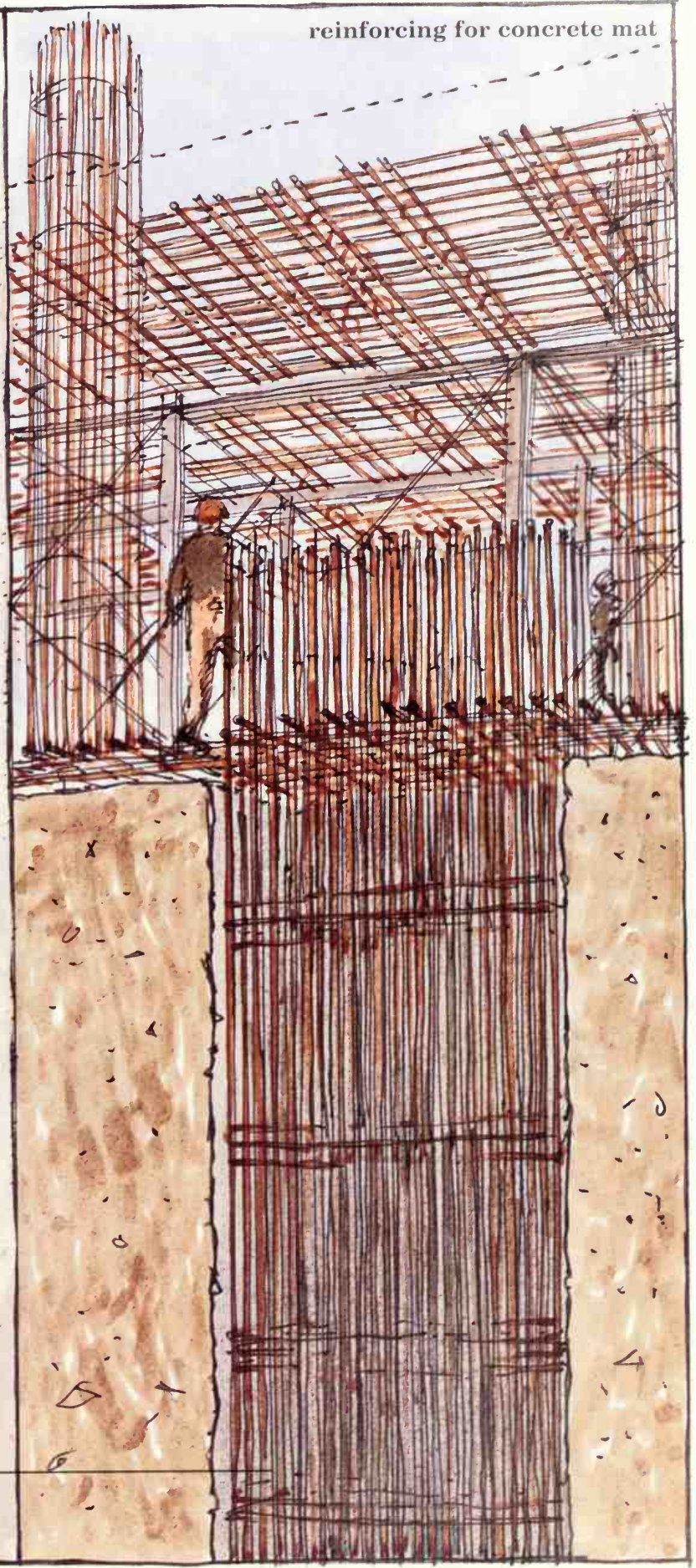
reinforcing for friction pile
