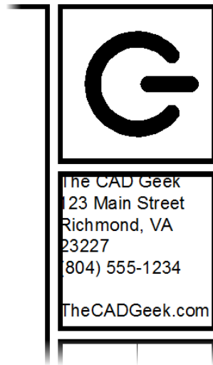
FIGURE 8.57: The company contact information placed within the title block before modifying formatting
