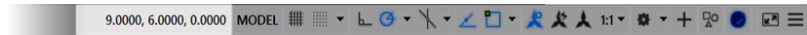
FIGURE 2.11: The x- and y-coordinates of the cursor are shown at the bottom of the AutoCAD window.
