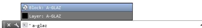
FIGURE 7.33: Inserting a block at the command line using an AutoComplete selection list
