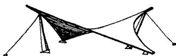
Wooden tent on timber-framed columns with steel cable stays, Bundesgarten Exhibition, Dortmund, architect: Behnisch, 1969.
