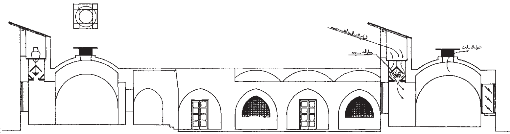
100. Ventilation system at girls' primary school
