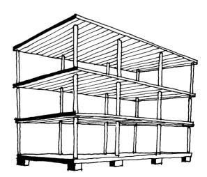
Figure 4.16 Column and slab structure facilitating 'open plan'.
