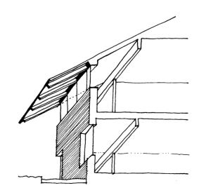
Figure 5.17 Clerestory/roof/wall junction.
