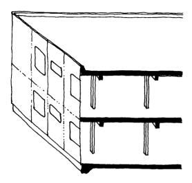
Figure 4.31 Cladding 'oversailing' structure.
