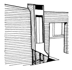
Figure 4.42 Ralph Erskine, Clare Hall, Cambridge, 1968. Rainwater chute.
