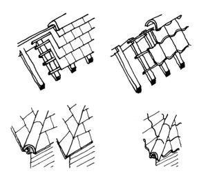
Figure 4.40 Traditional heavy slate and pantile roofs.
