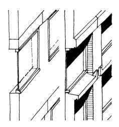
Figure 5.19 Flush/recessed fenestration.
