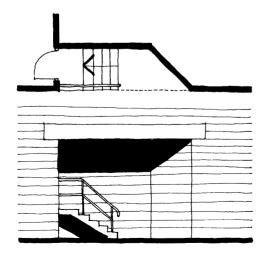
Figure 3.34 'Sub-space' off circulation route, plan/ elevation.
