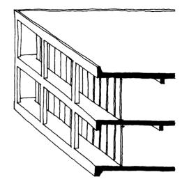
Figure 4.33 Cladding recessed behind structure.
