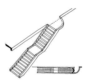
Figure 3.40 'Straight-flight' stair.
