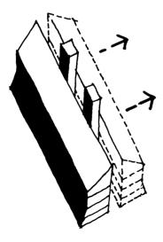
Figure 3.29 Linear plan, single/dual aspect.
