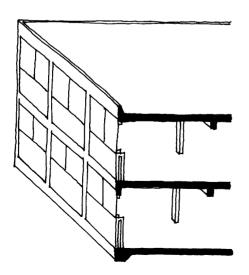
Figure 4.32 Cladding 'flush' with structure.
