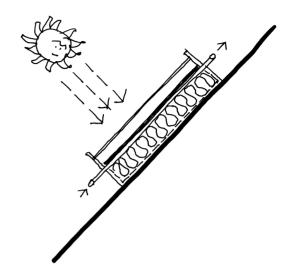
Figure 4.64 Flat plate solar collector.
