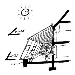
Figure 4.61 Direct solar gain.
