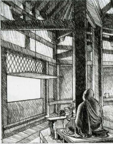
Outlook: Interior of Horyu-Ji Temple , Nara, Japan, A.D. 607 A window can be located such that a specific view can be seen from only one position in a room.
