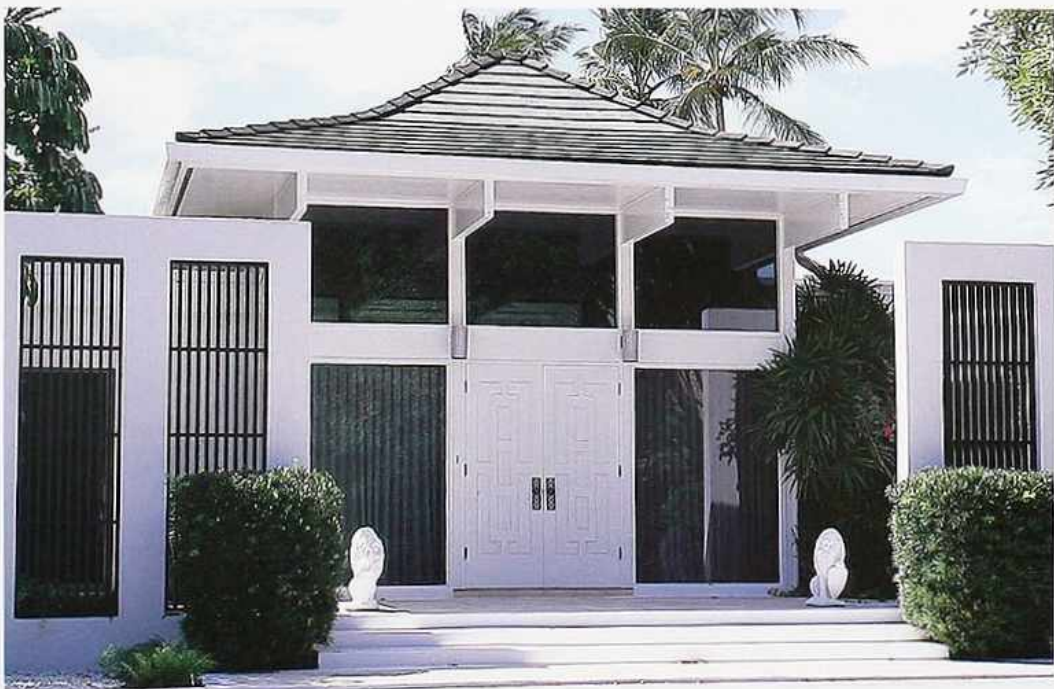
DW-89 Traditional Japanese post-and-beam-style entry with extended eaves, double flush doors, full glass side lights and lattice gates, modern house
