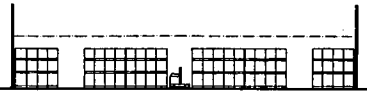
45 Reach fork-lift in block stack: 2.6 m aisle; 3.6 m stack height; 4.5 m building height (dotted)
