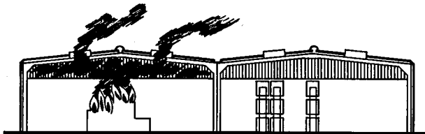
84 With vents and smoke reservoirs fire can be quickly contained and controlled
