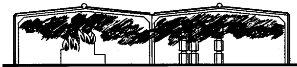
83 Factories without smoke vents can become rapidly smoke-filled, with fire spreading under roof surface
