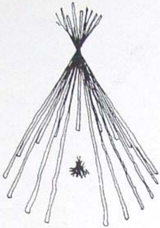
The structure of a native American teepee has an innate conical geometry, which produces a circular plan.
