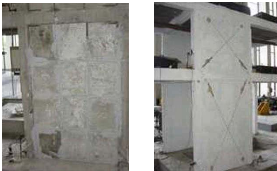
Figure 9. Completing the model (left); instrumentation installed (right)
