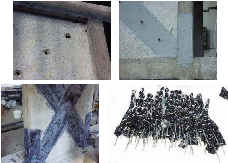
Figure 3. Specimen 2: Some details of CFRP incorporation
