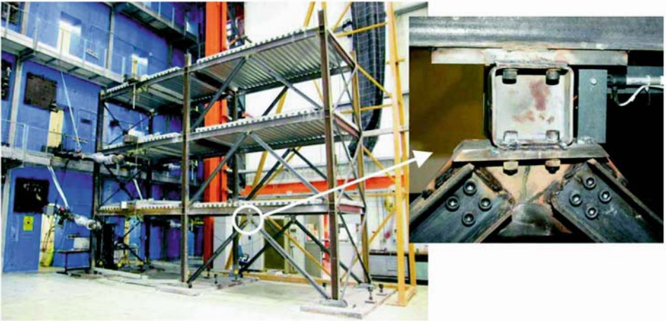
Figure 2. Steel frame mock-up at ELSA converted to a Hyde system using shear panel devices
