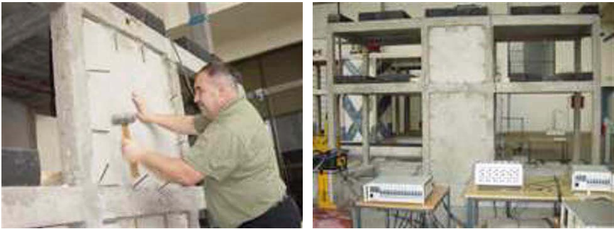
Figure 7. Specimen 3: Placing the anchor dowels (left); general view of the specimen after all anchor dowels are placed (right)
