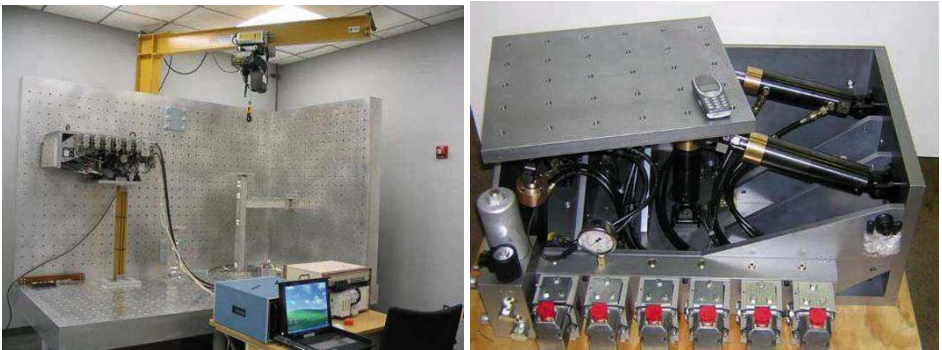
Figure 3. 1/5th scaled reaction wall and LBCB in the MUST-SIM facilities
