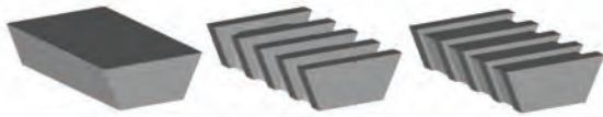
Figure 2: (a) Sloping façade planes; (b) sloping structure; (c) sloping structure and façade planes.
