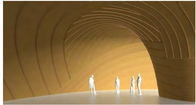
Figure 5: Geodesic D-strip models (in total five) which cover the interior of a freeform surface.
