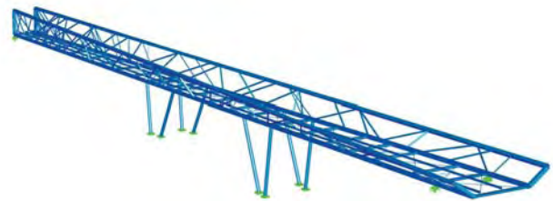
Figure 7: Irregular Latticed Girder
