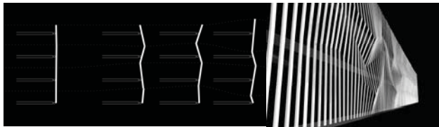
Fig.2: Initial Design Concept: a series of kinked beams create an overall surface with changing transparencies and patterns. The diagram shows possible sections through the construction shown in the rendering on the right.
