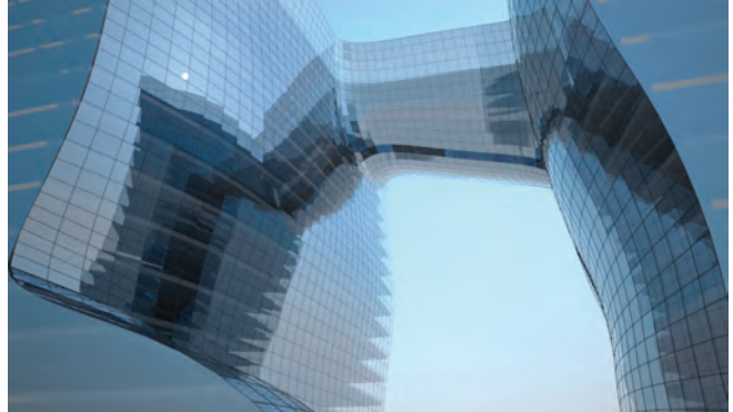
Figure 7: Rendered result of planarizing 'the Opus' - facade.
