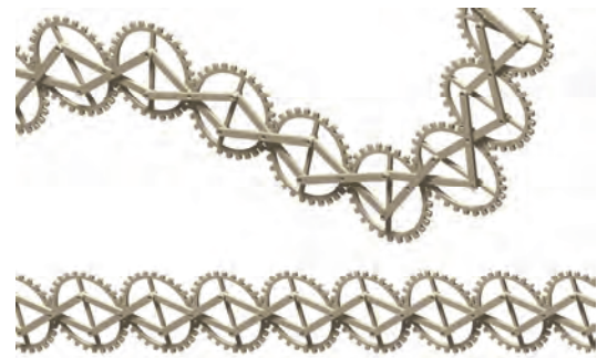
Figure 6: chain of elliptical gears, any 2D curve can be subdivided in this way and will be foldable
