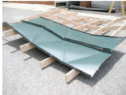
Figure 4- Standing seam test on frame
